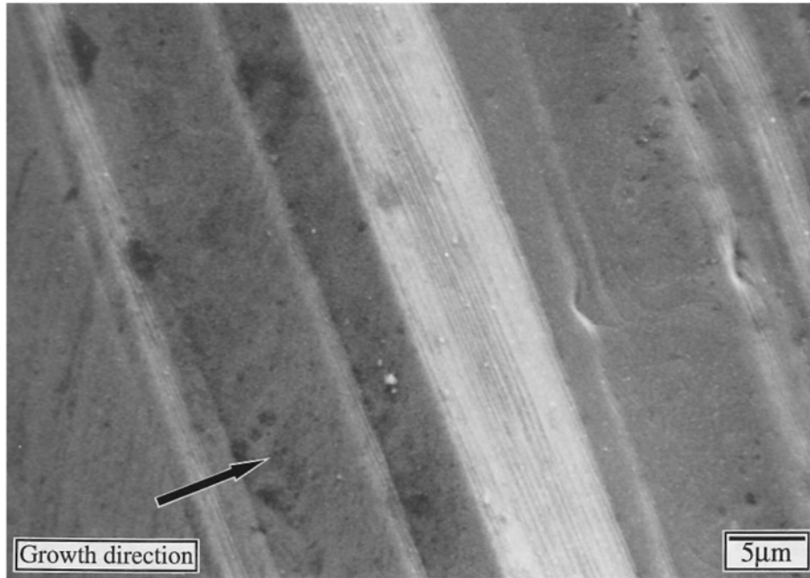
Fig. 5. A high magnification SEM micrograph showing the structure of growth facets.
