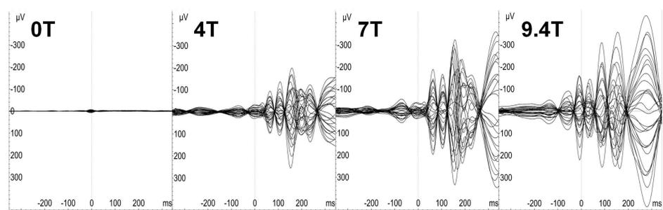
Figure 1. Pulse artefact at different magnetic fields. EEG signal is averaged around the heart-beat event
