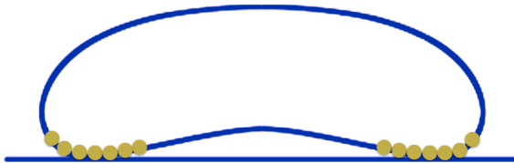
Figure VI.9: Schematic view of a large Leidenfrost drop with beads in it. The beads quickly occupy the neck region where the drop evaporates the most.
