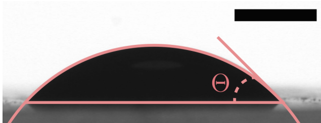
Figure I.1: Photography of a drop on a glass slide. The scale bar represent 1 mm.
