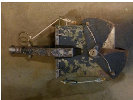
Figure 2-14: Benne à main Eckman (A. Donnay)
