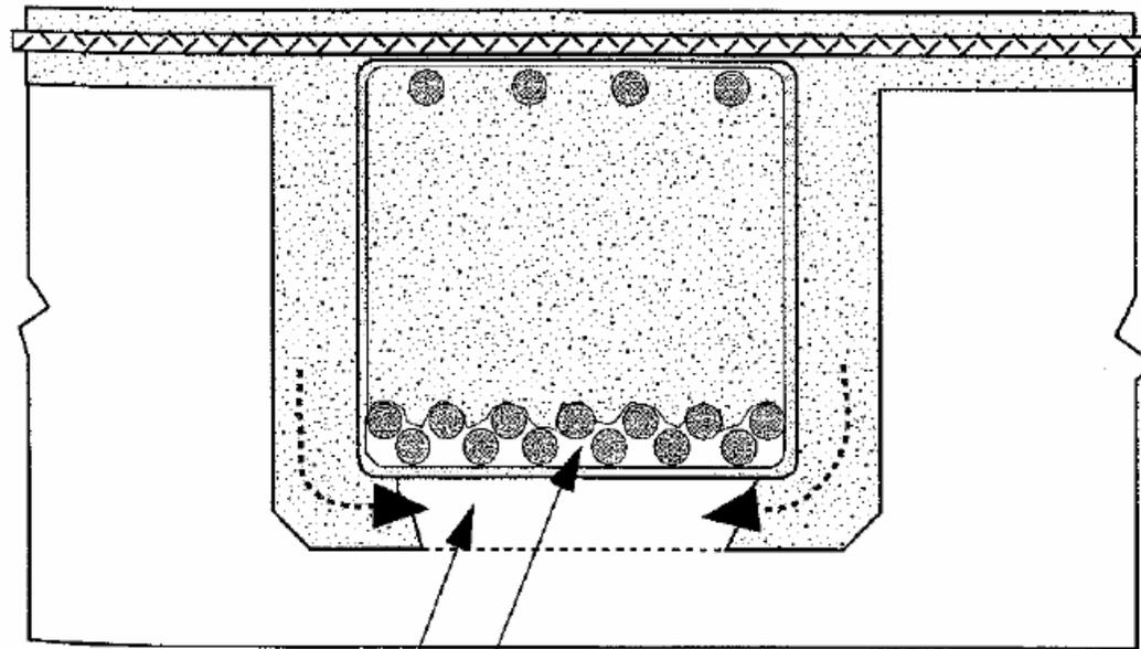
Congested reinforcement prevents concrete from filling around bars.
