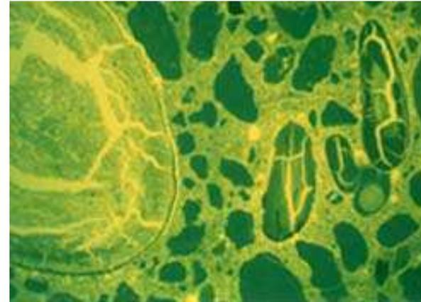
*Internal and external cracks caused by ASR in porous chert (RBL-DK).*
