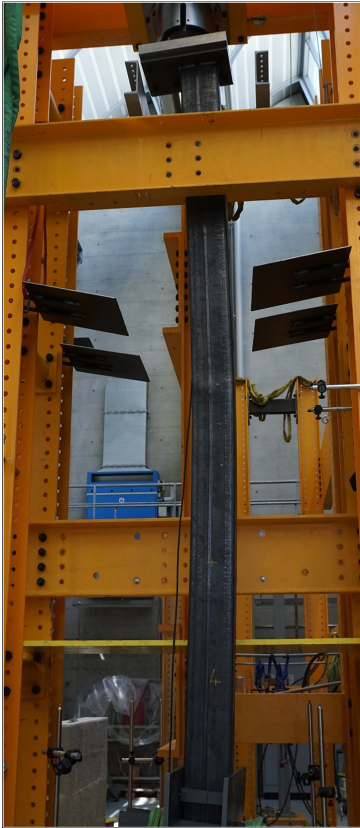
Buckling specimen after test
