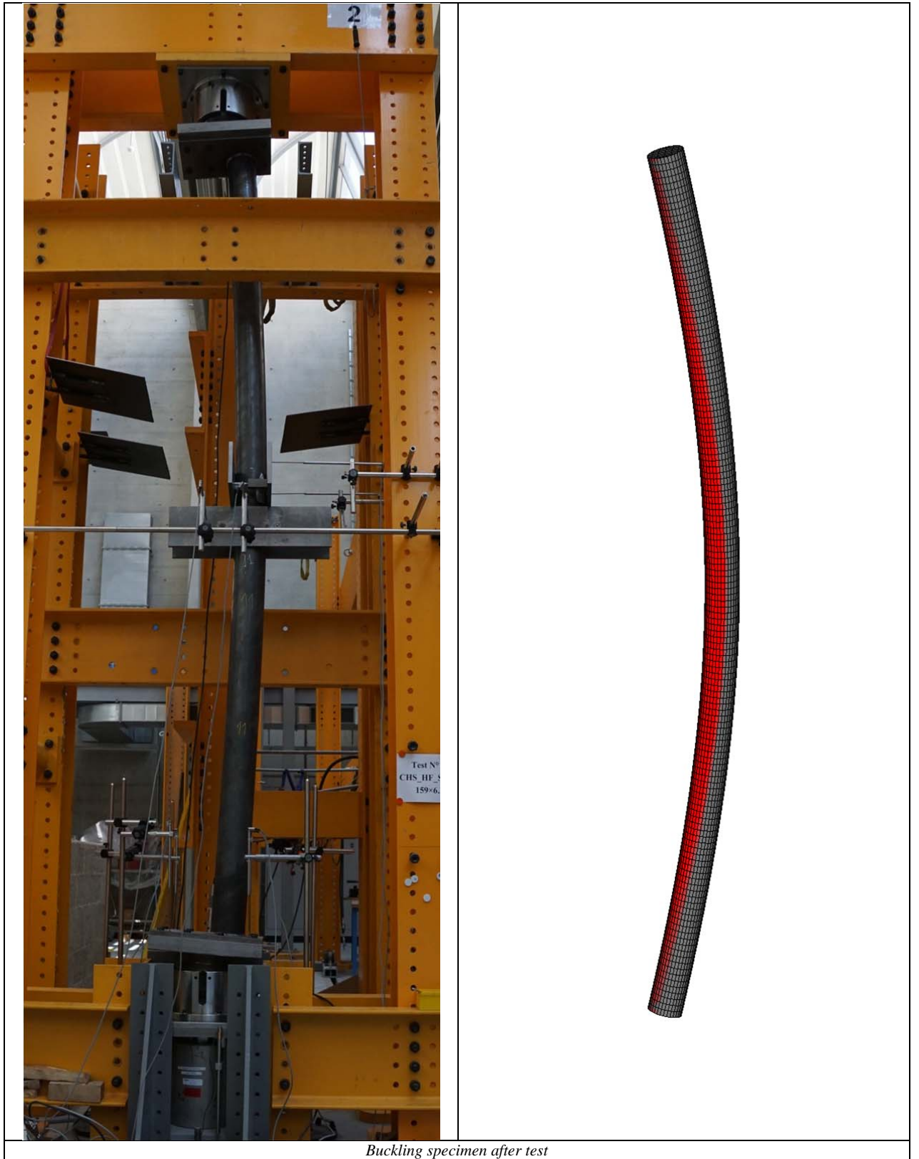
Buckling specimen after test
