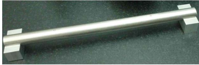
Figure 55 – Invar' bar with 100 mm basis
