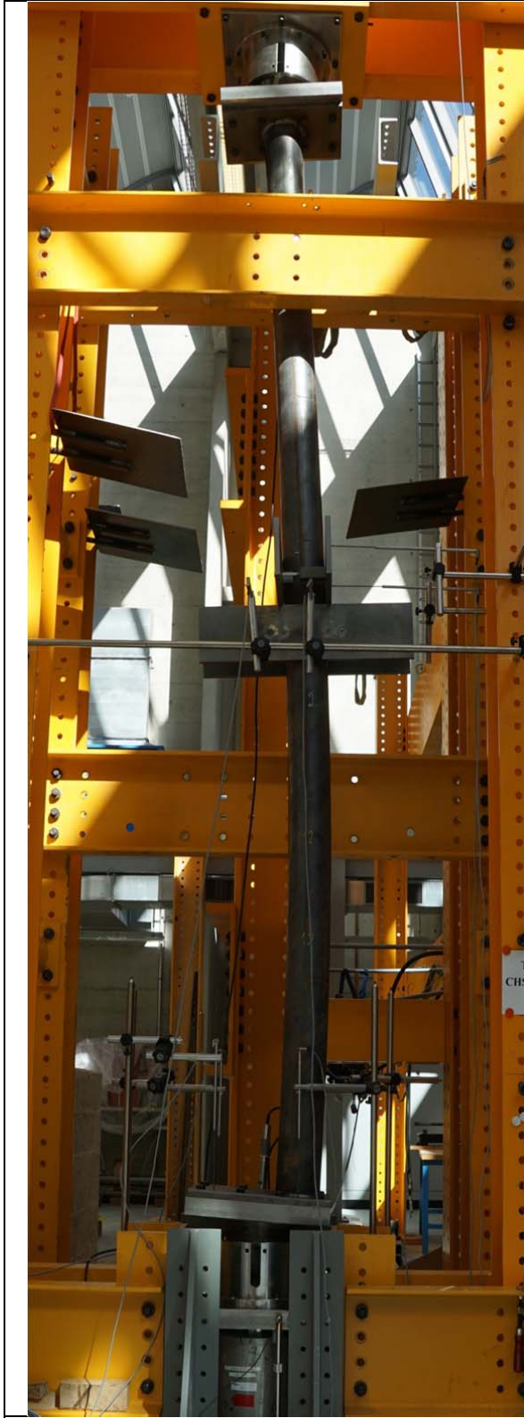
Buckling specimen after test
