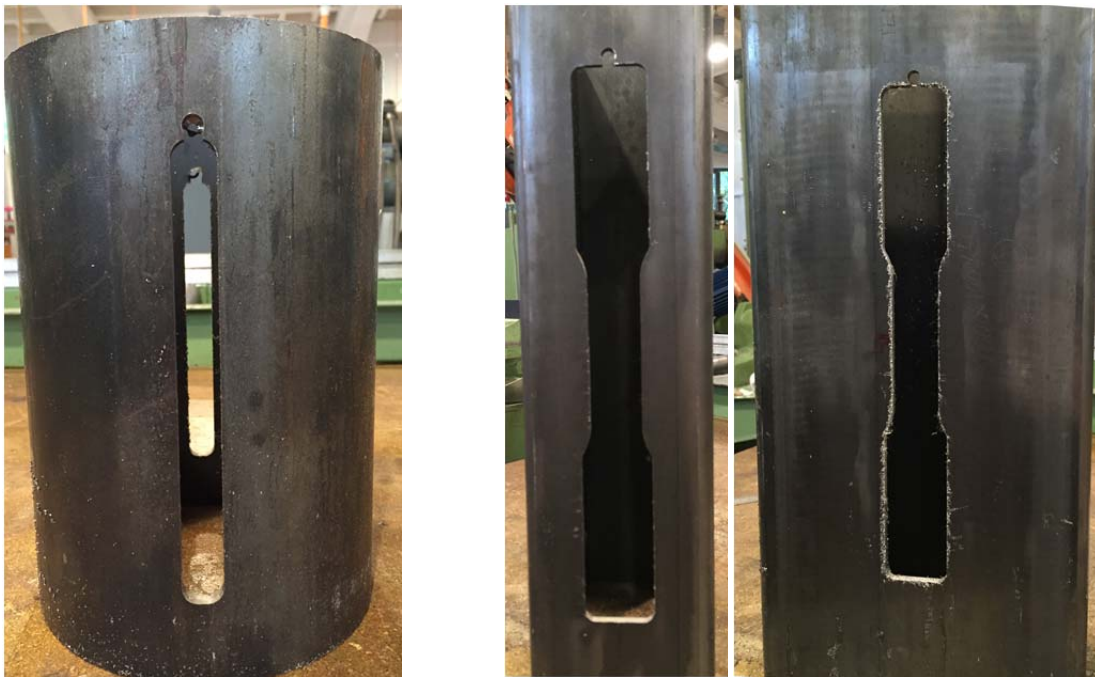
Figure 23 – Extraction of coupons from – a) CHS sections – b) RHS sections
