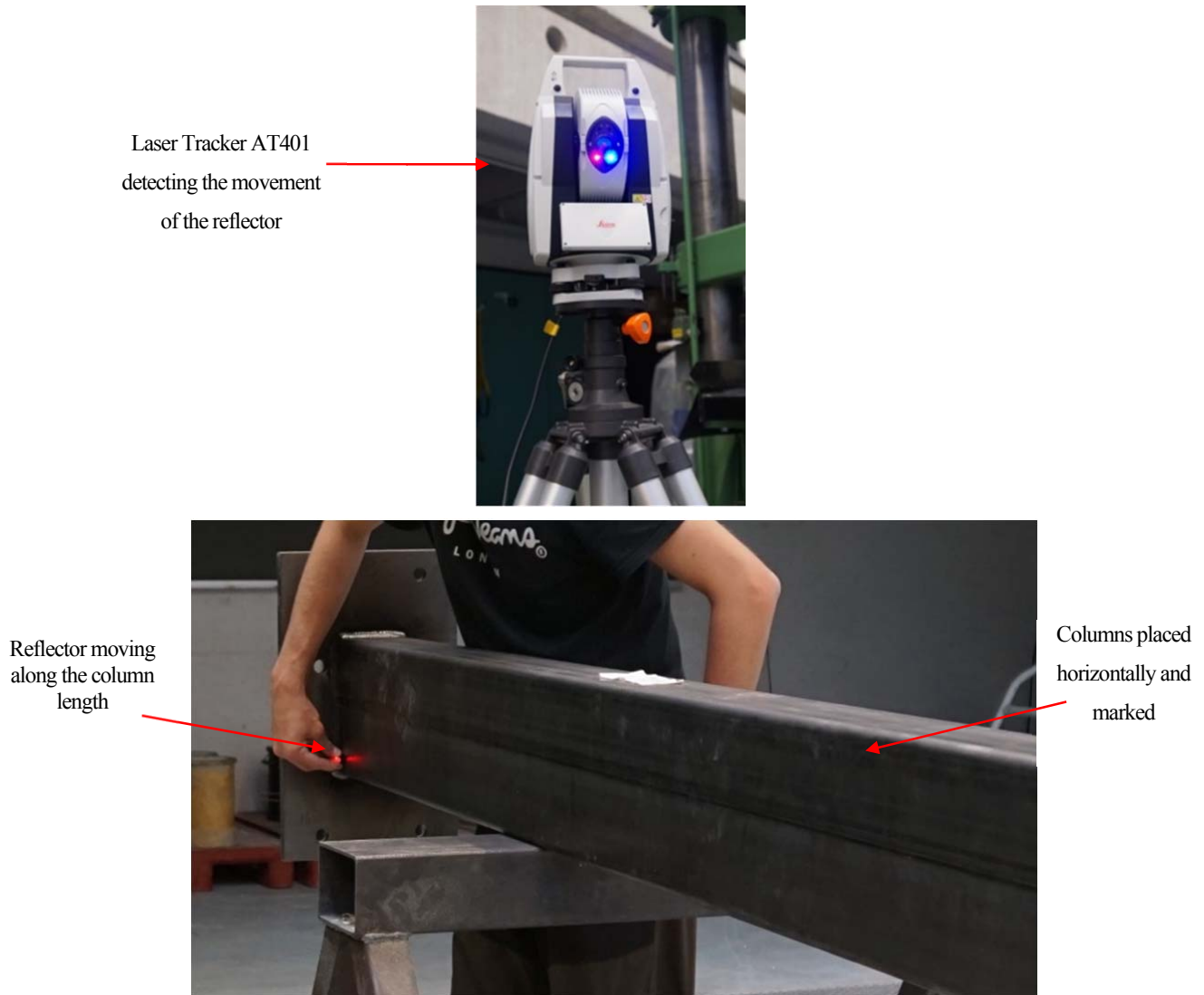
Figure 47 – Measurement of geometrical imperfections – Topometric procedure
