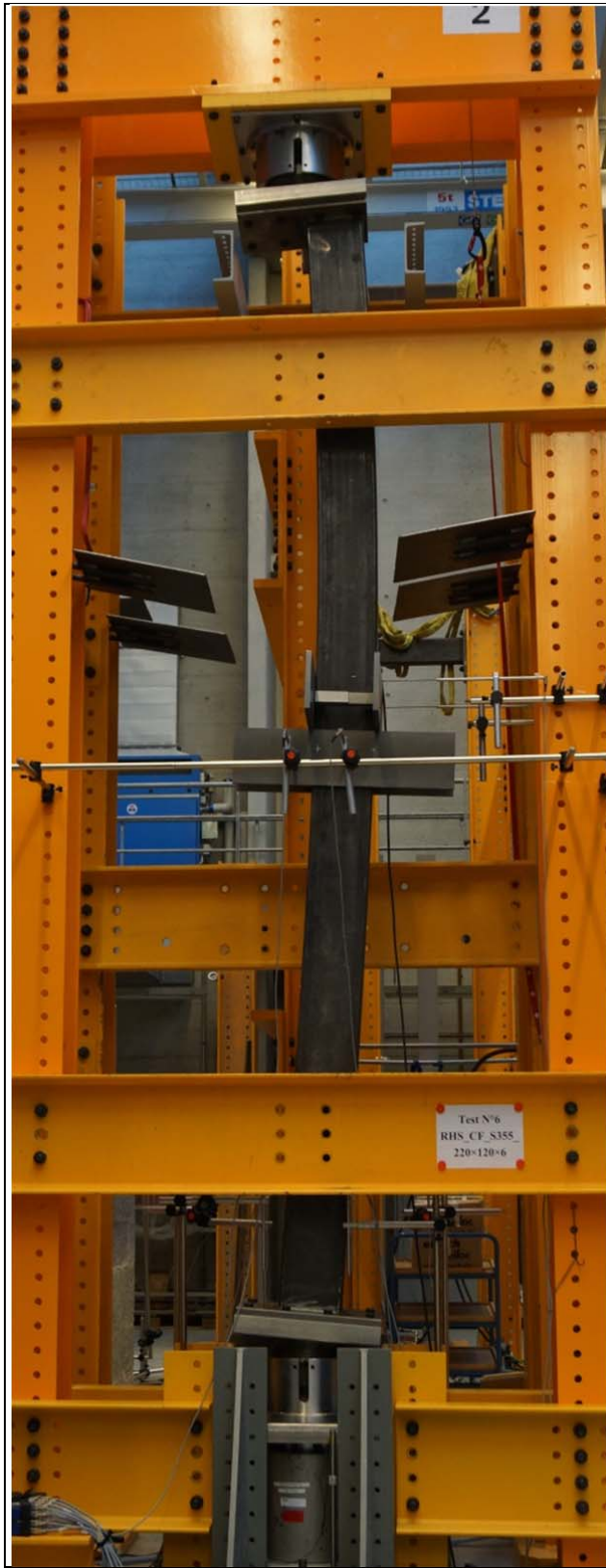
Buckling specimen after test
