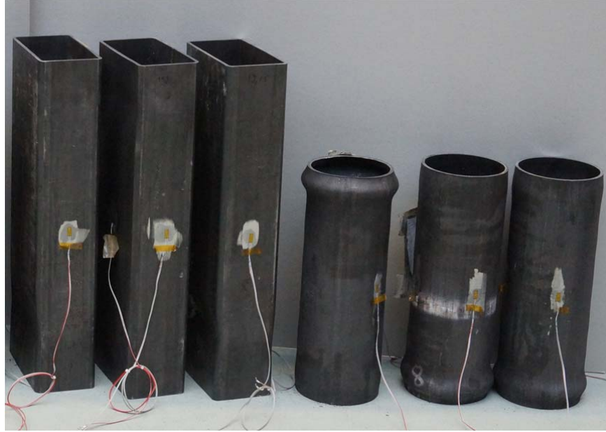
Figure 63 – Failure shapes of all stub columns
