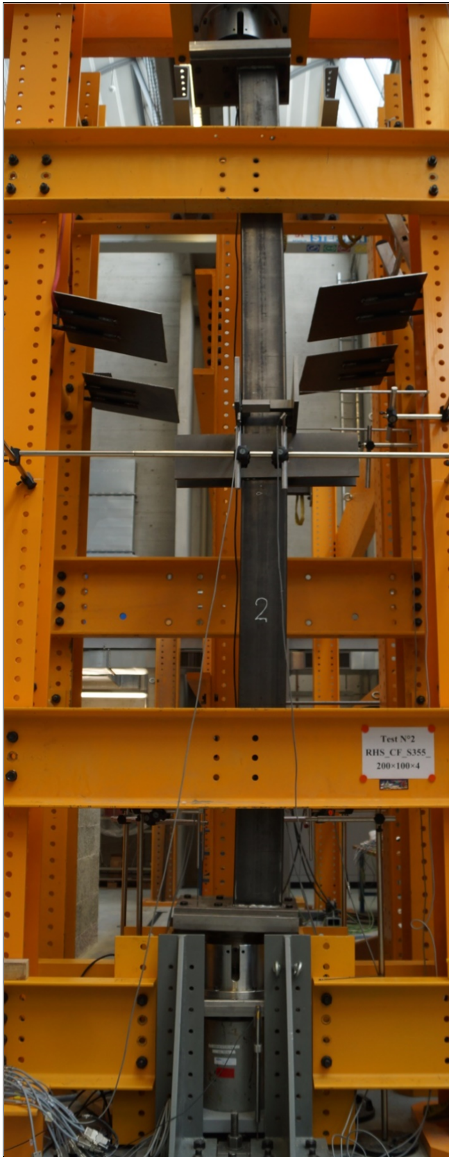
Buckling specimen after test
