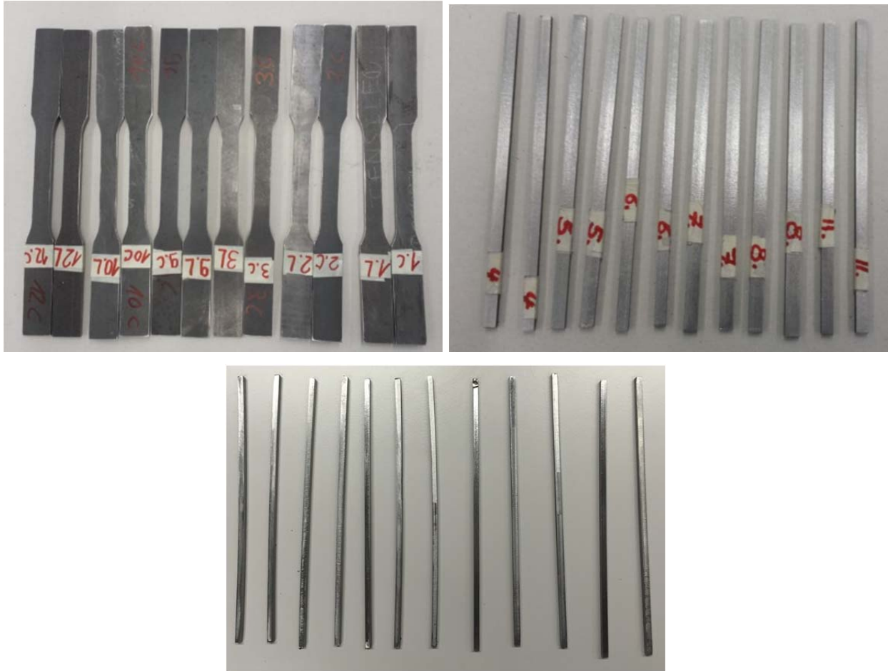
Figure 24 – Tensile coupons extracted from – a) flat faces of cold-formed RHS sections – b) corners of cold-formed RHS sections – c) corners of hot-rolled CHS
