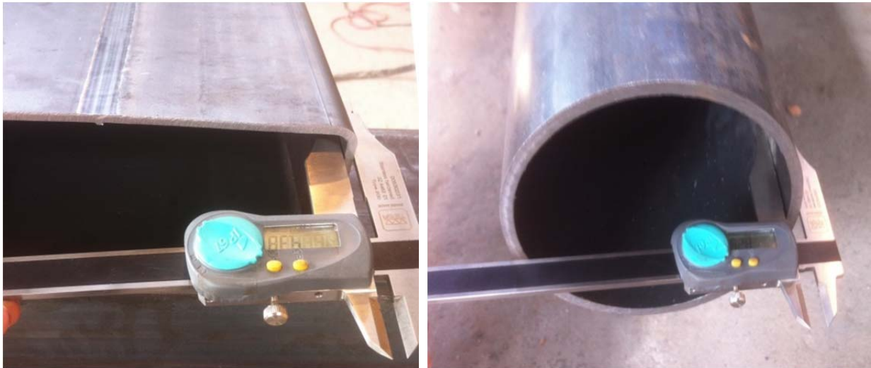
Figure 19 – Measurement of cross-section dimensions of circular and rectangular sections
