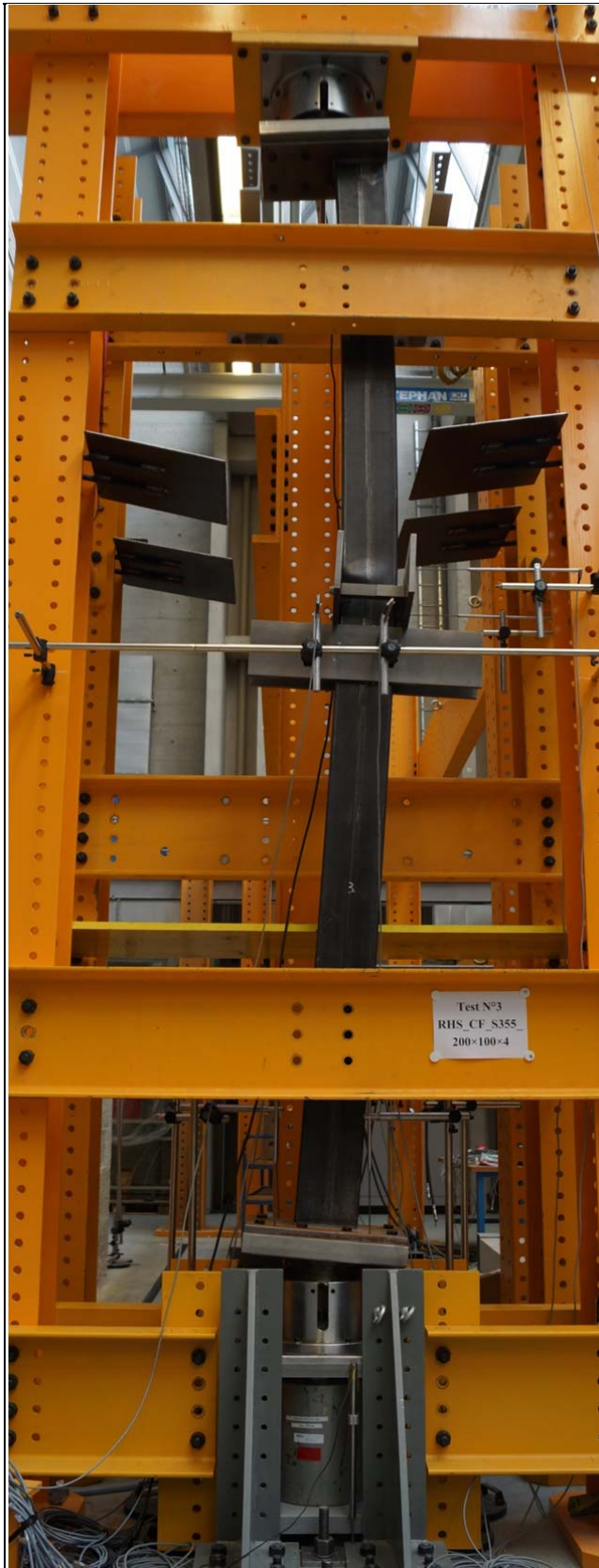
Buckling specimen after test
