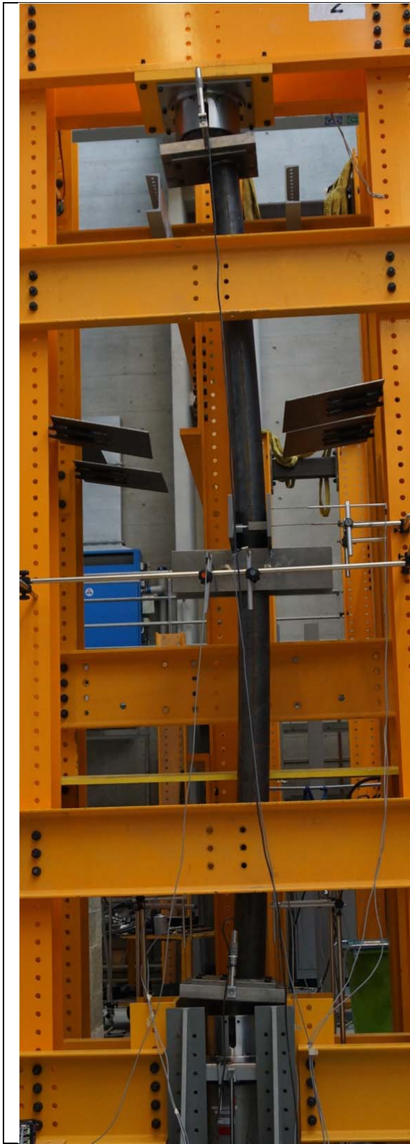
Buckling specimen after test
