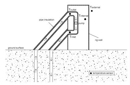
Figure 3 - Temperature sensors location during the DTRTs
