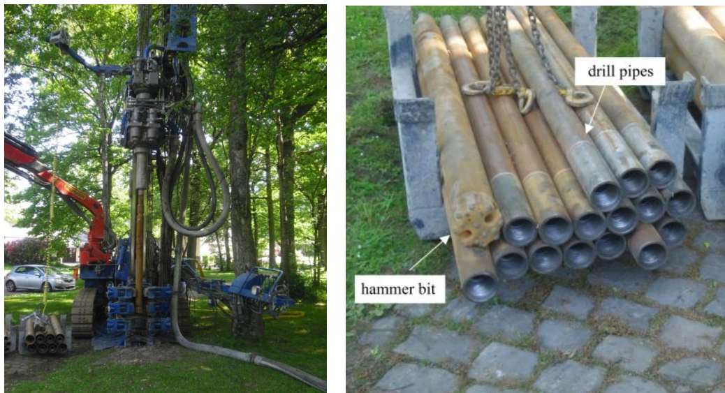
Figure 2.2 -Drilling rig (left) and drill pipes (length of 2 m, outer diameter of 13.5 cm) (right)
