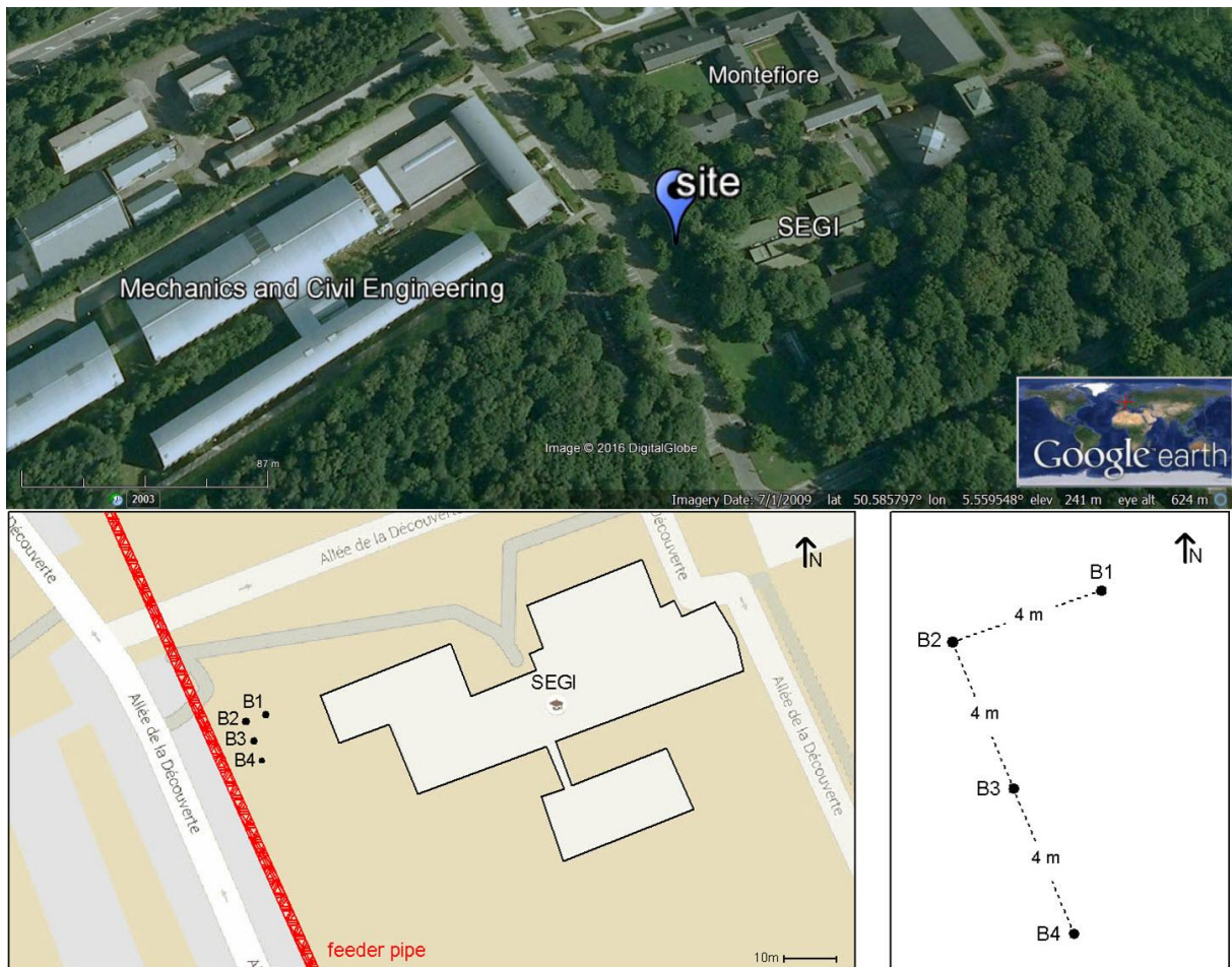
Figure 2.1 - Site location on the campus of the University of Liege (retrieved from Google Earth©) (red line: heating feeder pipe, SEGI: General Service of Informatics, B1 to B4: four BHEs)
