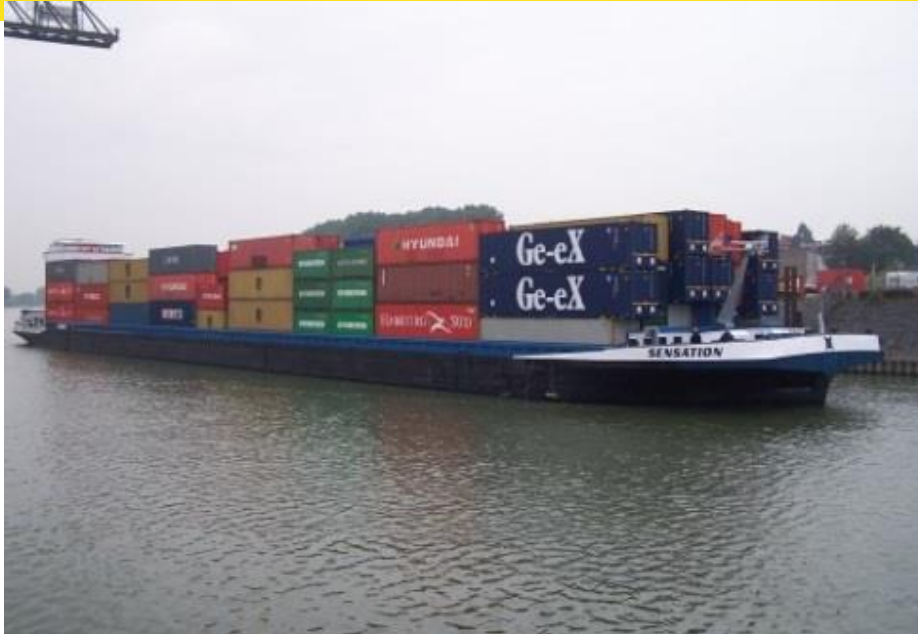
Newly built containervessel (135 x 17.10 m.), partly loaded with high cube containers.
