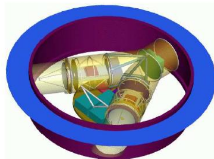
Figure 2.3: Cutaway of LISA's instrument [8]. The actual spacecraft will be protected with a cover.
