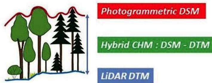
Figure 37: Hybrid Canopy Height Model. Adapted from Bonnet (2009).
