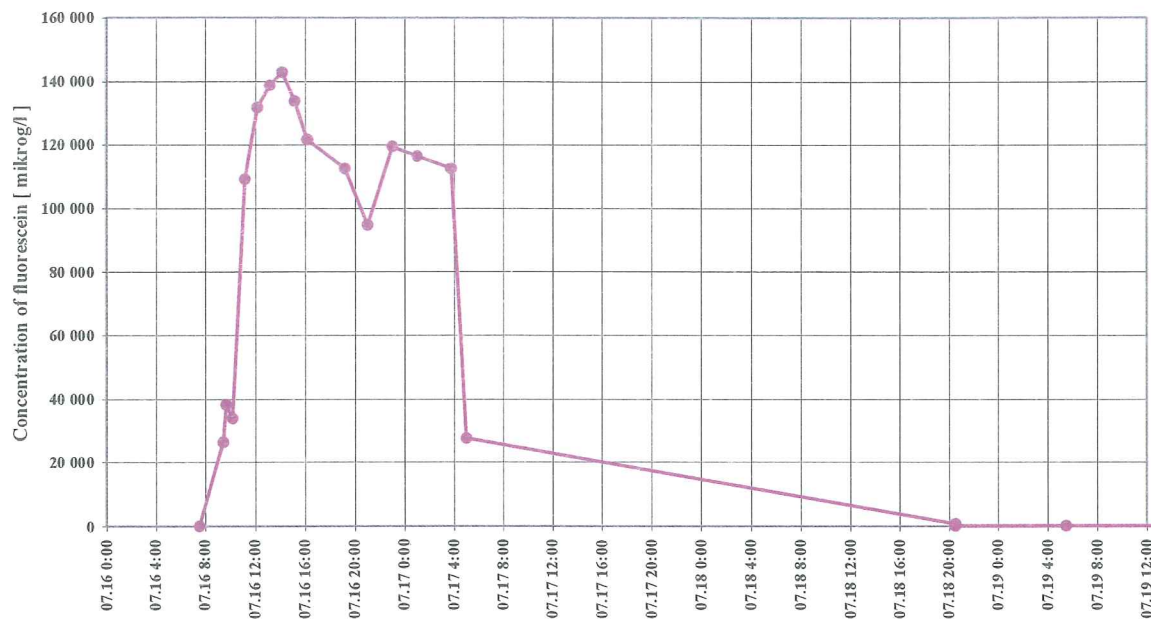
Fig. 4 Tracer test, Szatmárcseke No.1, fluorescein in No.5 (tracer)-well. Fluorescein analysis: Laboratory in Eger.
