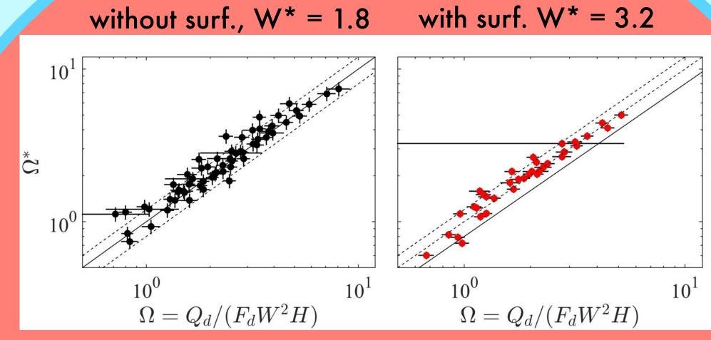
Parity plot of measured dimensionless droplet volume  $\Omega$  vs. empirical law :
