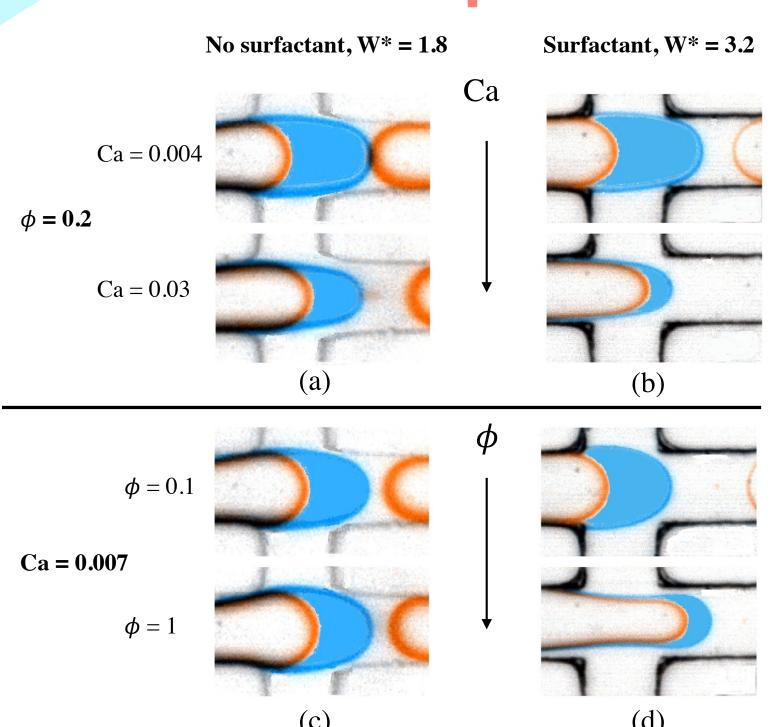
Superposition of two snapshots from the same experiment right after pinch-off and initial retraction (orange) and after T1 at the end of the inflation step (blue).
