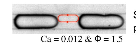
Satellite droplet looping in the horizontal plane between two main droplets.
