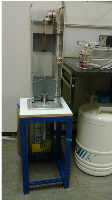
Figure 3.12: Experimental setup for temperature-dependent measurements. The vertical position of the sample holder above the Dewar tank containing the liquid nitrogen controls the temperature.
