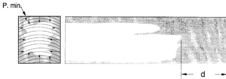
Figure 35. Measure of minimal lateral (P.min), mean lateral and minimal longitudinal (d) penetration of copper sulphate in wood samples (adapted from CEN/TR 14734 (2004)).
