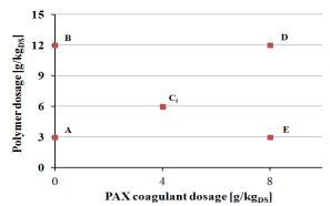
Fig. 1. Design of experiments representation.
