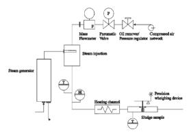
Fig. 2. Scheme of the convective micro-dryer.
