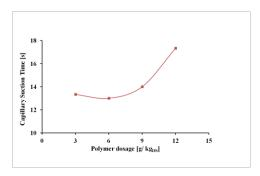
Fig. 3. CST results on activated sludge
