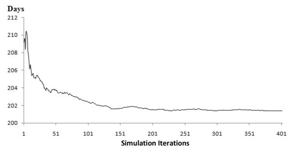
Fig. 2: The convergence test showing the minimum number of simulation runs required for installing 72 OWTs
