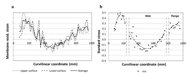
**Fig. 13.** (a) Membrane strain on the two surfaces & average strain in the sheet pile 2: after cooling, in the longitudinal direction, (b) normalised longitudinal residual stress in the sheet pile 2: after cooling, in the longitudinal direction.
