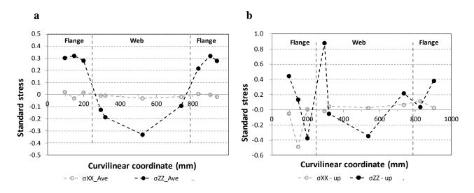
**Fig. 9.** (a) Average residual stresses in the sheet pile 2, after cooling, in two directions: X and Z, (b) residual stresses in the sheet pile 5, after cooling and straightening, on the upper surface and in two directions: X and Z.
