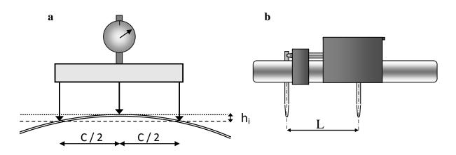
Fig. 11. Equipment used to measure the deformations due to sectioning: (a) deflectometer, (b) extensometer.
