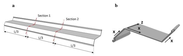
**Fig. 3.** (a) Localisation of the measures: XRD and ring core method in section 1 and sectioning method in section 2 (L= 6000 mm), (b) global reference frame.
