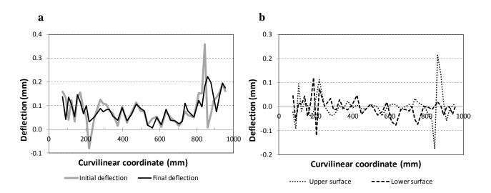
**Fig. 12.** (a) Deflections on the upper surface, before and after sectioning, (b) difference in the deflection before and after sectioning the samples, on the upper and lower surfaces.
