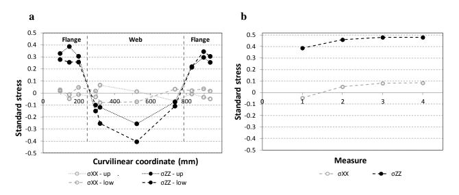
**Fig. 8.** Residual stresses in sheet pile SP2, after cooling: (a) on the upper and lower surfaces in two directions: X and Z, (b) verification of the stress reproducibility in the left flange, on the upper surface and in two directions: X and Z.
