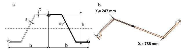
**Fig. 2.** (a) Sheet pile geometry (AZ 38-700+1, b= 700 mm, h= 501 mm, t=19 mm, s= 14.2 mm,  $\alpha$ = 63.2°, length= 6000 mm), (b) location of curvilinear coordinates: X<sub>c</sub>.
