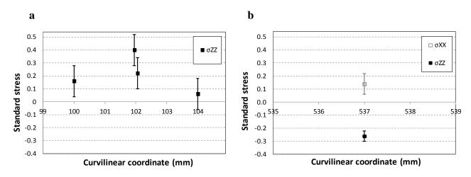
**Fig. 5.** Normalized residual stresses by the XRD method and error bars: (a)  $\sigma_{ZZ}$  in sheet pile SP2, after cooling, on the left flange (b)  $\sigma_{ZZ}$  and  $\sigma_{XX}$  in sheet pile SP5, after cooling & straightening, on the web.
