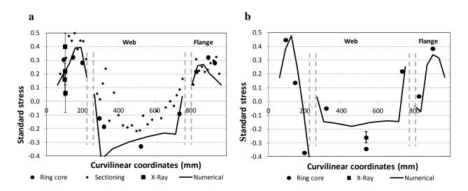
**Fig. 15.** Comparison between experimental and numerical longitudinal residual stresses: (a) in sheet pile SP2, after cooling, (b) in sheet pile SP5, after cooling and straightening.
