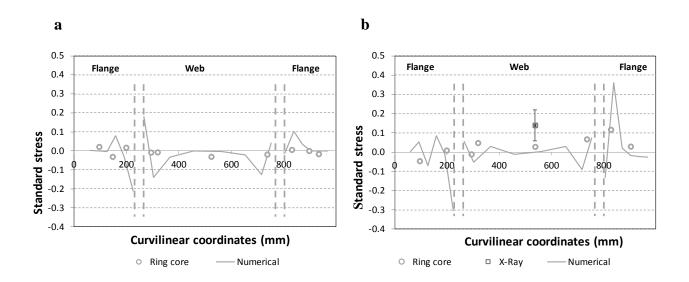
**Fig. 14.** Comparison between experimental and numerical transverse residual stresses: (a) in sheet pile SP2, after cooling, (b) in sheet pile SP5, after cooling and straightening.
