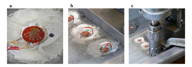
**Fig. 6.** (a) Strain gauge rosette sticked on the sheet pile surface, (b) strain gauge rosettes after holes drilling, (c) ring drilling procedure.
