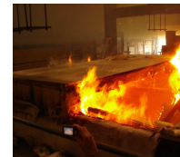
Timber floor tested in horizontal furnace
