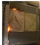
Facade tested in vertical furnace
