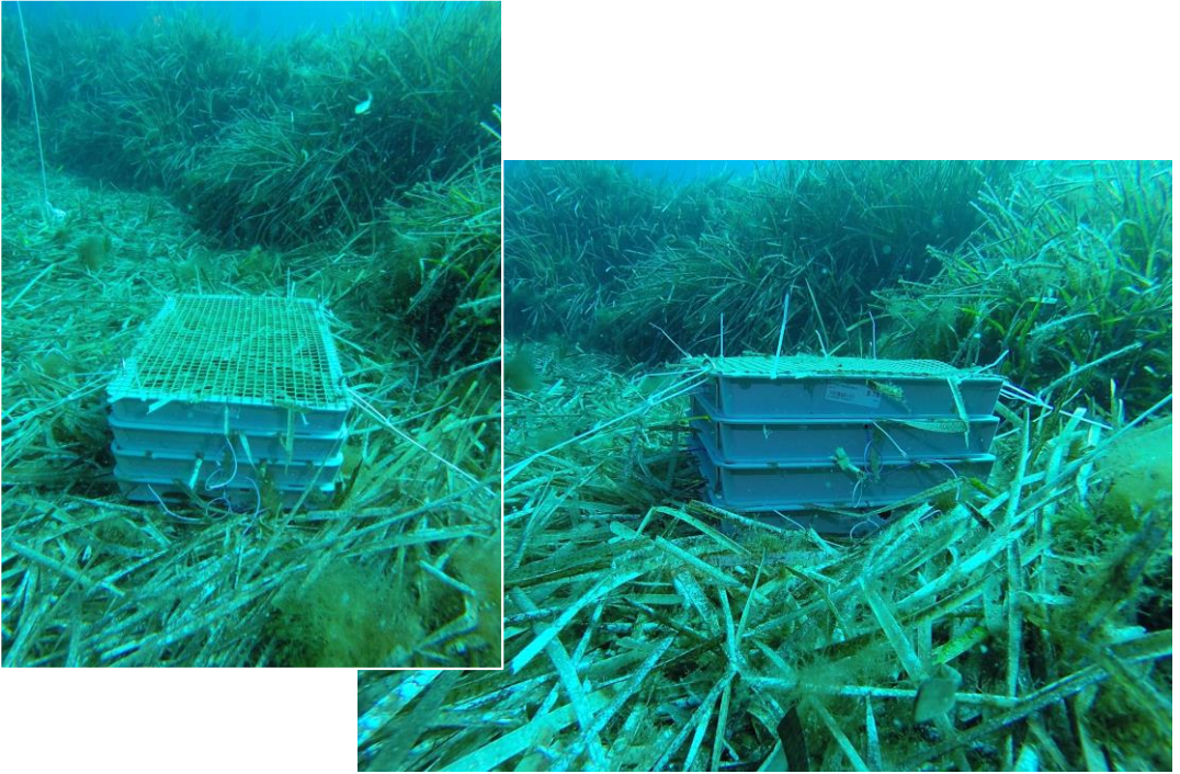
Figure 4.1: Design of the experiment, showing the 4-layers construction inside the HARBOR-site EMA. This figure shows the design in “open configuration” at the beginning of the experiment with the 10 mm sieve on the top layer. The figure shows the steel poles and lines used to prevent any movement during the 48h experiment.
