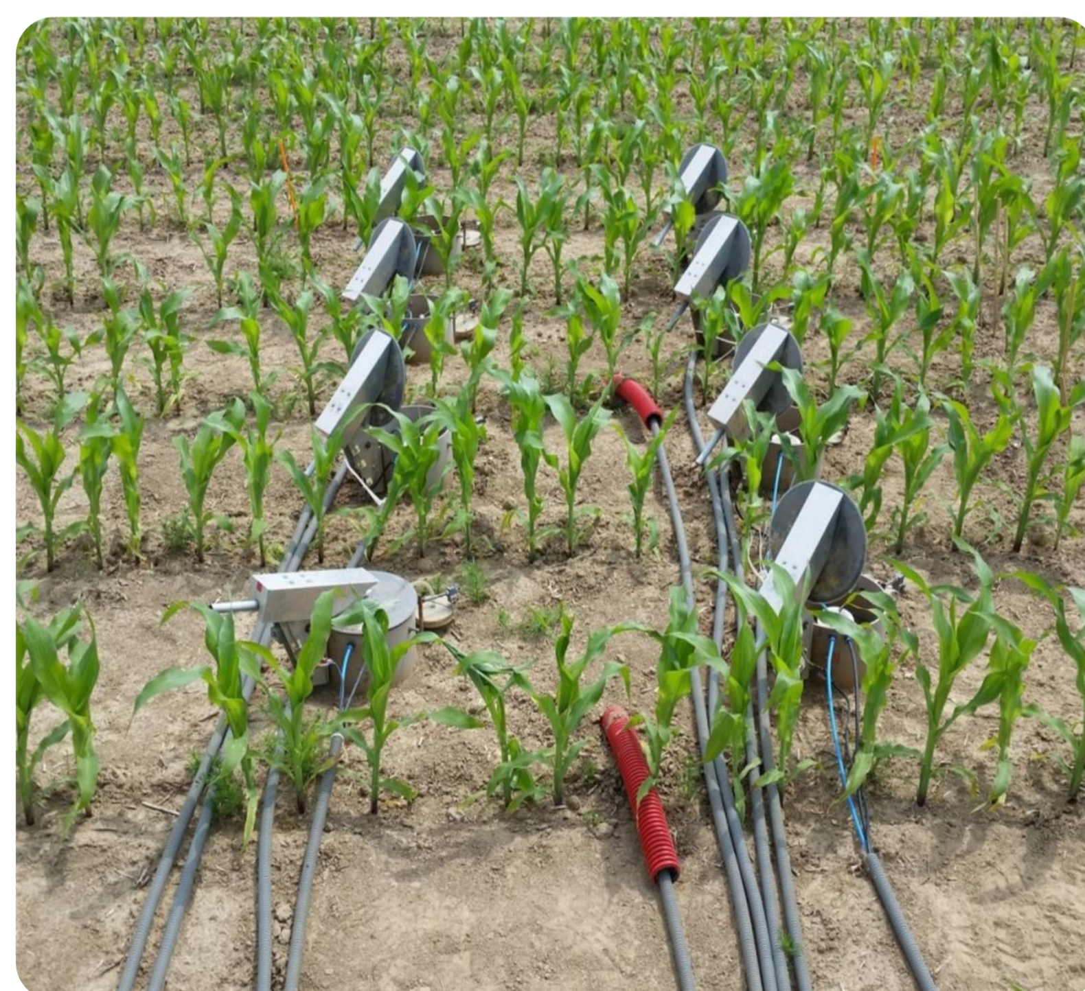
Fig. 1: Automated dynamic closed chambers: PVC collars + motorized lids + air circulation to gas analyzers (Gascard® NG OEM CO 2 analyzer and Thermo Scientific™ 46i N 2 O analyzer:). 8 chambers per treatment were used to continuously measure CO 2 and N 2 O fluxes at a 4.5-hour resolution.
