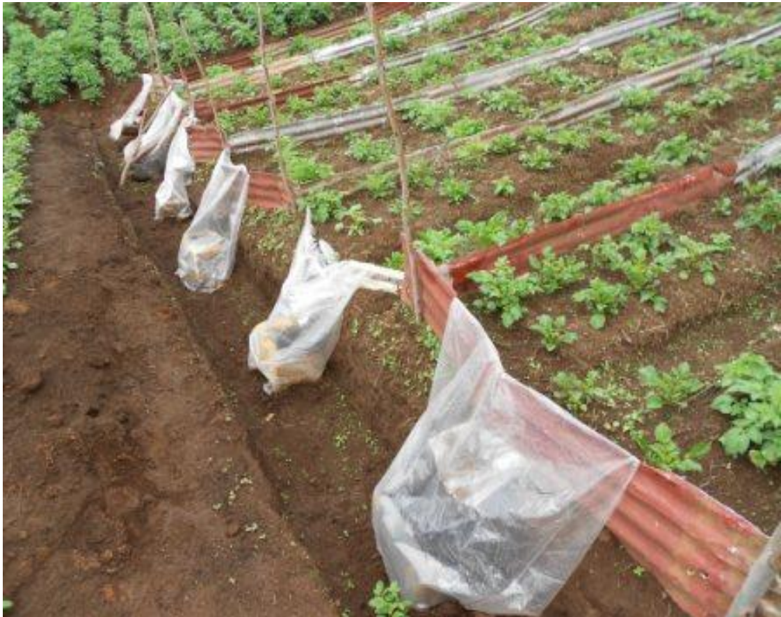
Figure 4-3 Device for water and sediments collection
