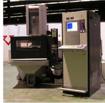
Figure 10. Picture of the EDM from ONA™ (spark erosion)
