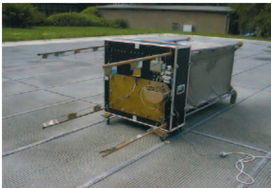
Fig. 12: Picture of the GTO on a test-site and the CONCEPT equivalent for simulations
