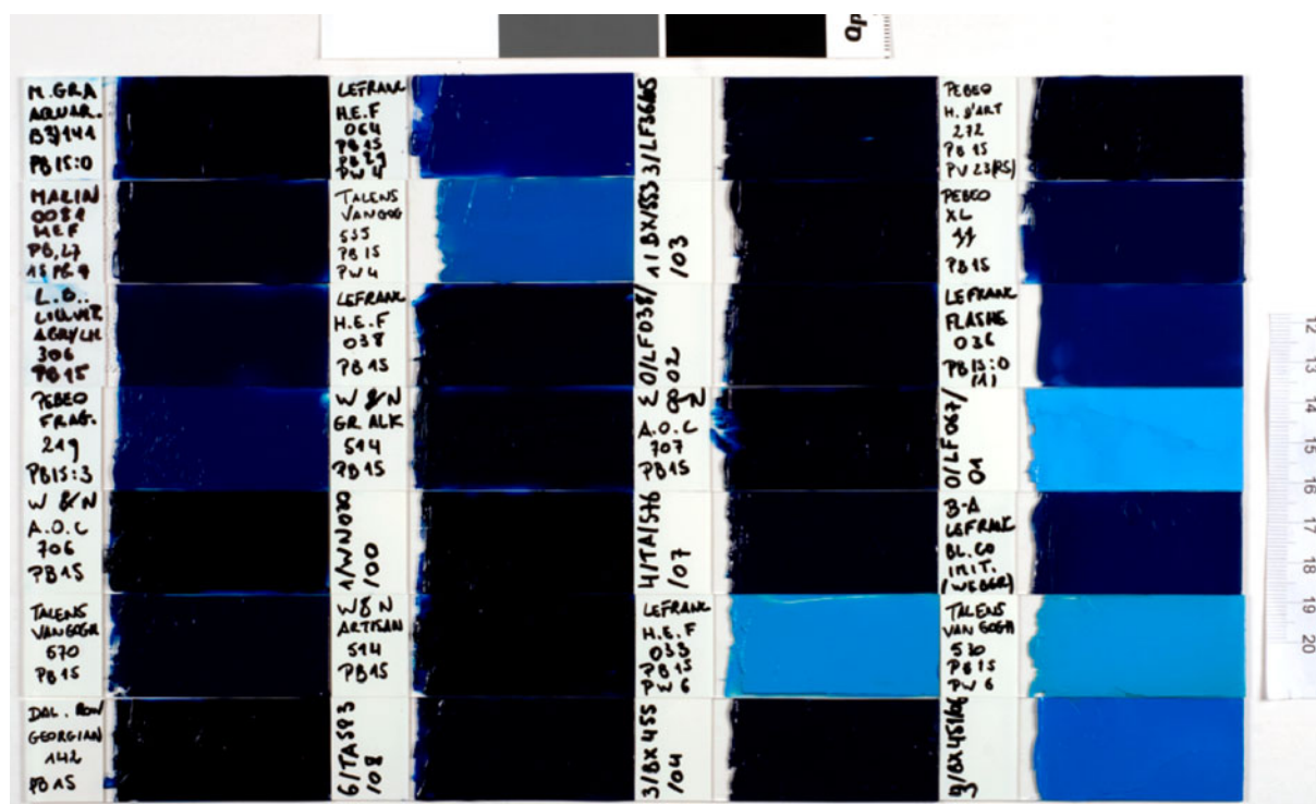
Figure 4: Dried paint films obtained from various commercial phthalo blue-based paints on glass slides. Figure taken from Defeyt 2 .
