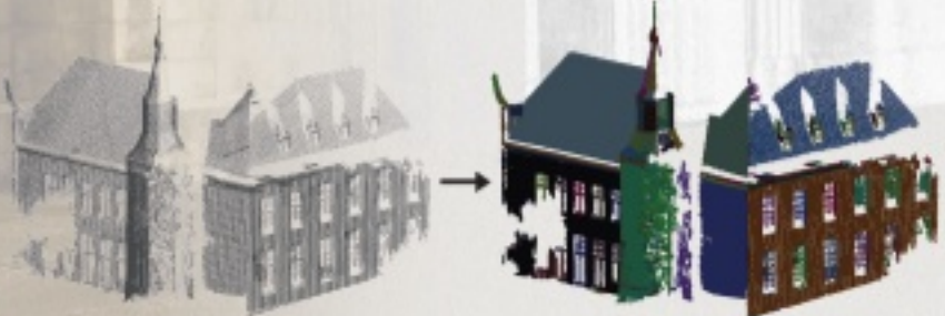
Segmentation of a 1 Billion point Cloud representing the Colonster Castle (Liège)
