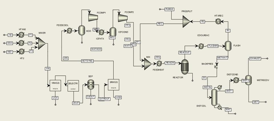
Sub-processes linked through 2 stages-compression with intermediate cooling.
