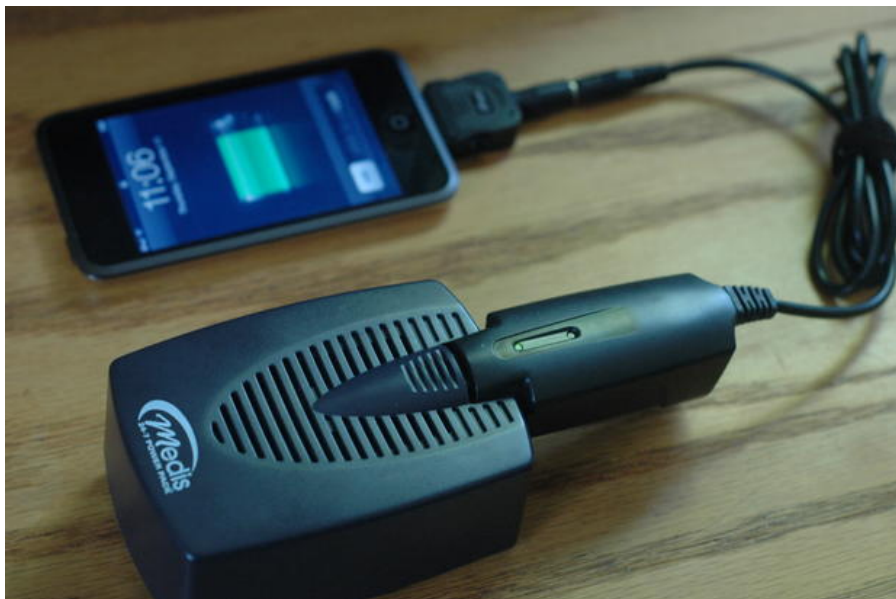
Figure 10: 'Medis 24-7 Power Pack' DBFC charging a smartphone. Reproduced from the website of CNET [47]. Martin LaMonica/CNET News.
