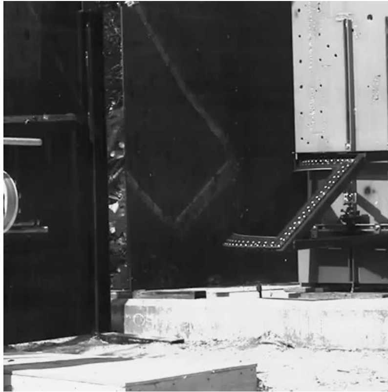
Bird strike on a wind shield test
