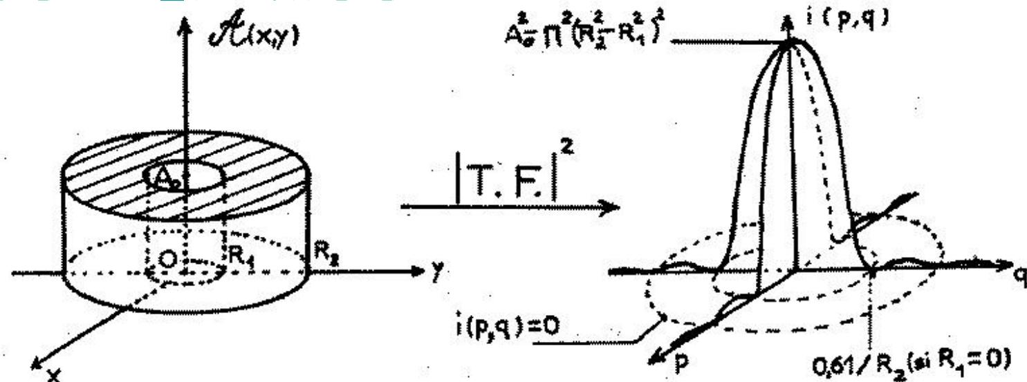
$$i(\rho') = |a(\rho')|^2 = (A_0 \pi)^2 [R_2^2 2 J_1(Z_2) / Z_2 - R_1^2 2 J_1(Z_1) / Z_1]^2, \quad (8.1.8)$$
