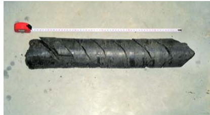
Figure 5.24: Fracturing pattern in a core taken from the borehole 2001-2 [Bastiaens et al., 2003].
