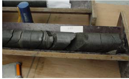
Figure 5.23: Fractures observed in the clay core taken from a borehole drilled out of the gallery, as shown in Figure 5.22 [Bastiaens et al., 2003].
