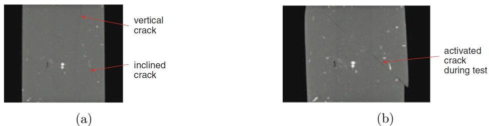
Figure 5.15: X-ray CT vertical sections through the specimen BCTIMODAZ02: (a) Before the test. (b) After the test; after [Bésuelle et al., 2014].
