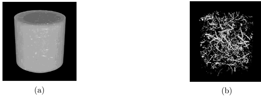
Figure 5.14: Illustration of the pre-existed inclusions in Boom Clay sample BCTIMODAZ02 before the test. (a) X-ray CT 3D reconstruction of the surface of specimen. (b) X-ray CT 3D reconstruction of the inclusions inside the specimen [TIMODAZ, 2010b].
