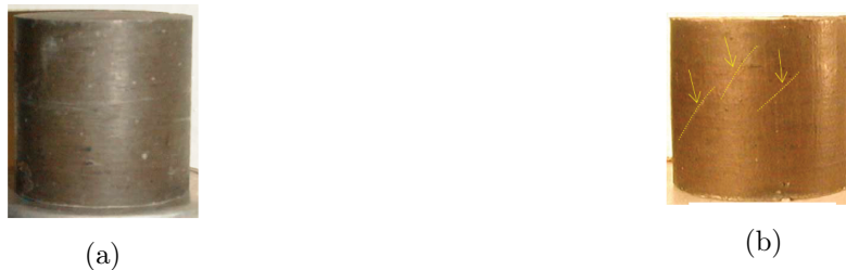
Figure 5.6: Representation of the sheared samples after the test: (a) EXP Coll 1. (b) EXP Coll 2 [Coll, 2005].
