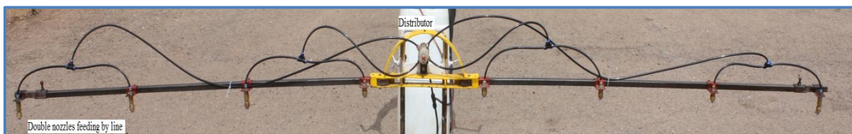
Figure 53: Parallel boom design with double nozzles feeding from upstream (distributor) to downstream (tip nozzle) points
