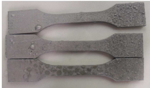
Figure 1: Deterioration of the samples' surface following solutionizing heat treatment at 530°C for 6 hours.
