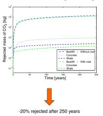
Back to the shaft sealing considering a coal seam 0,25m wide above the injection zone.
