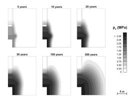
Figure: Evolution of gas pressures in the different materials during CO<sub>2</sub> storage in the coal mine.
