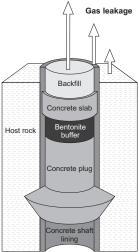
Figure: Layout of the sealing system used for the shaft n<sup>o</sup>6 of Anderlues coal mine.
