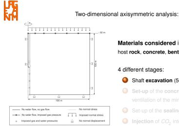
Figure: Geometry and boundary conditions used for the hydromechanical analysis.
