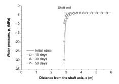
Figure: Evolution of pore water pressure profiles in the shale during the shaft excavation.
