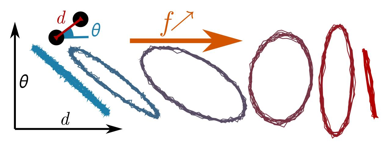
Modes can be out of phase  $\to$  **non-reciprocal** motion. Necessary for low Re swimming!
