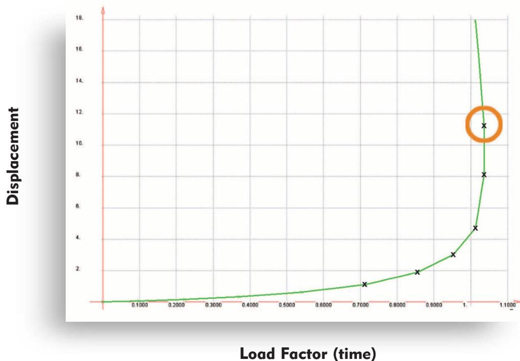
Figure 4: Displacement of a node as an illustration of the collapse.
