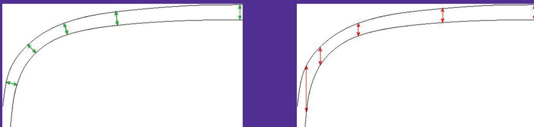
Figure 5: Vertical vs. orthogonal gaps on load-displacement curves.
