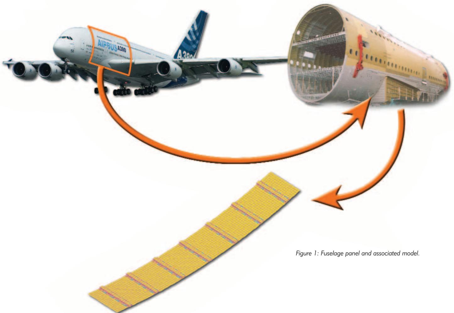
Figure 1: Fuselage panel and associated model.
