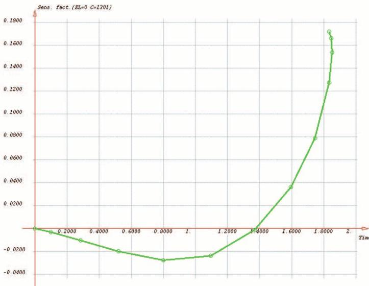
Figure 6: Sensitivity of load factor with respect to ply thickness.
