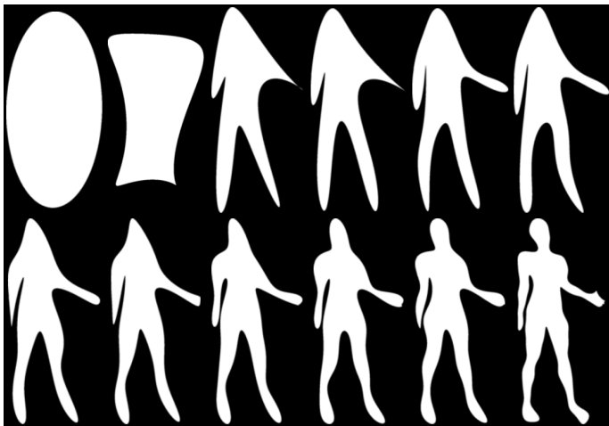
Figure: Approximations of a human silhouette by an increasing number of Fourier descriptors.
