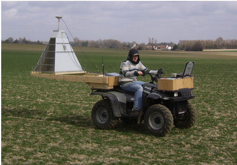
Figure 3.5: All-terrain vehicle holding the GPR system constituted of a horn antenna linked to a vector network analyzer, the DGPS device and the PC. Picture taken on the 23 th of March 2009 in a barley field near Walhain, Belgium.
