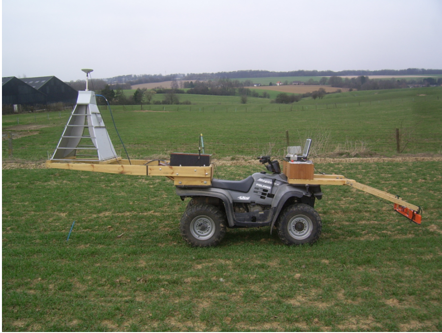
Figure 4.2: All-terrain vehicle holding the GPR system constituted of a horn antenna linked to a vector network analyzer, the DGPS device, an EM38 sensor and the PC. Picture taken on the 15 th of March 2010 in a Burnia near Louvain-la-Neuve, Belgium.
