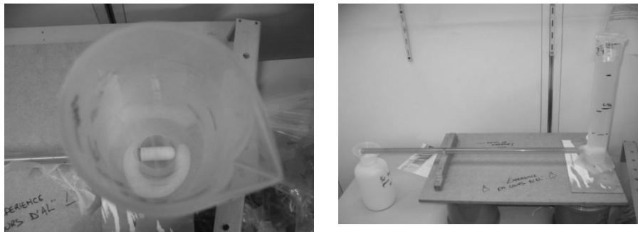
Figure B.1 the ceramic cup lysimeter is inserted tightly into the column where the realistic soil solution is added to increasing Si concentrations.
