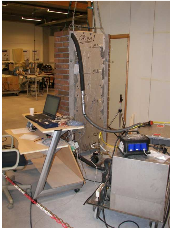
Photo 3: Back site of collector with cool water unit, circulation pump and temperature sensors
