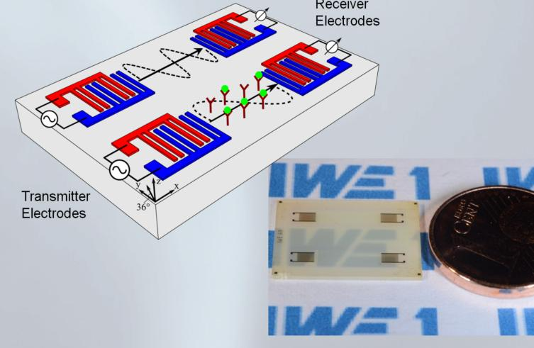
When a probe (e.g. proteins) is being deposited, the change in the frequency of the acoustic waves can be measured
