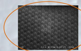
The silicon micropillar array works as an autonomous capillary pump, capable of transporting a specific amount of bio-samples into the sensing area without pumping external requirement.
