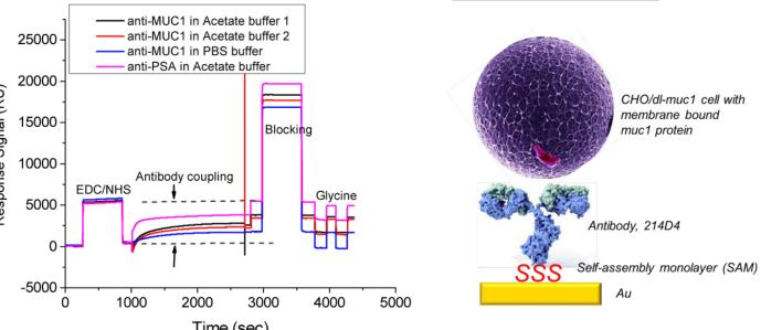
Successful Anti-MUC1 antibody coupling on gold surface (monitored by SPR) via mixed "COOH" and "OH" SAM
