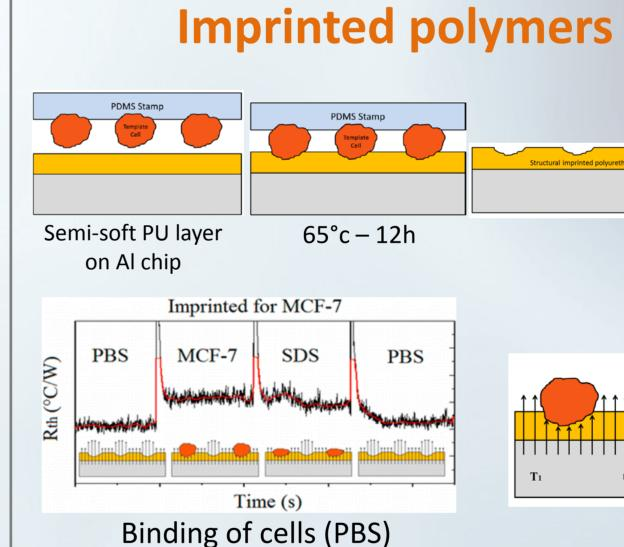
Sensor set-up for heat-conduction measurements ( $T_1 = 37.0$ °C) Patent application: WO2012/076349A1  $\rightarrow$  cell lysis (SDS)  $\rightarrow$  rinsing (PBS)
