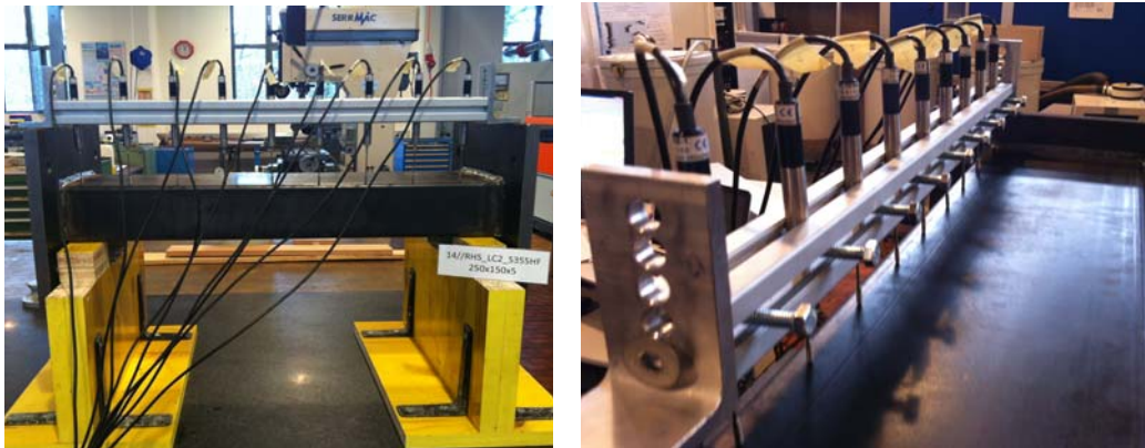
Figure 55 – Geometrical imperfections measurement – LVDTs detail.
