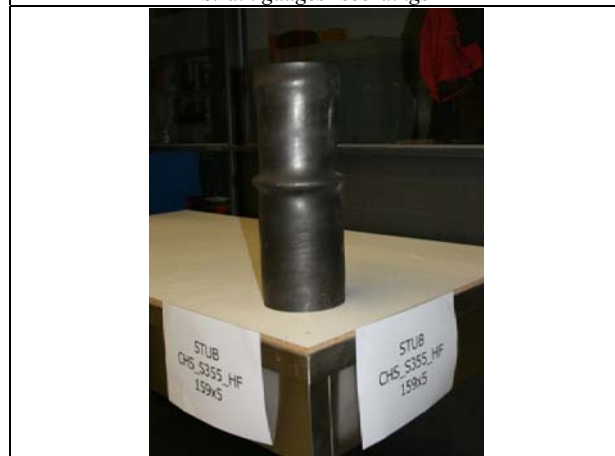
Local buckling failure Exp test VS. FE test
