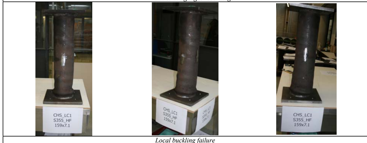
Local buckling failure
