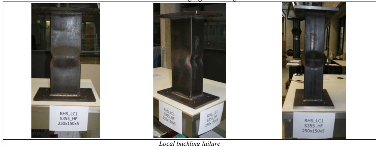
Local buckling failure
