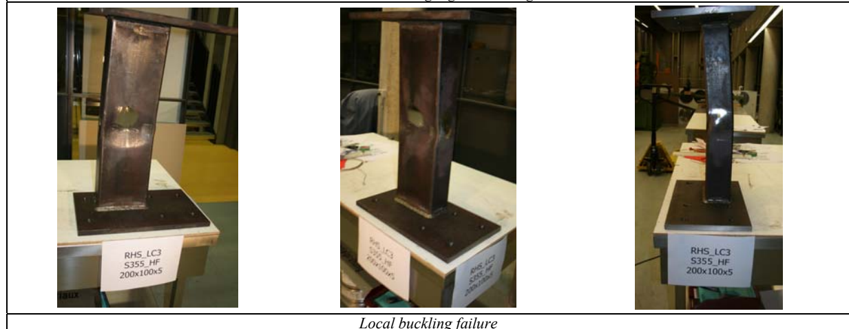
Local buckling failure
