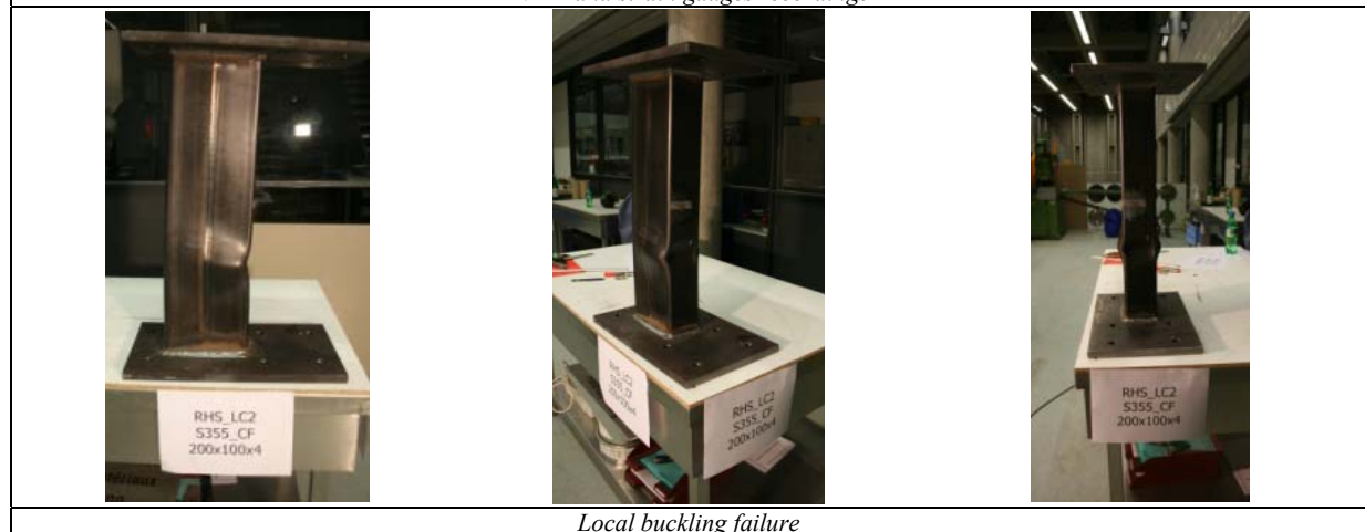
Local buckling failure
