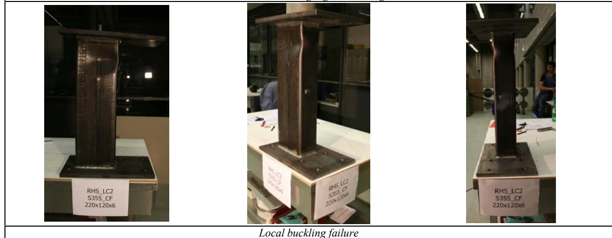
Local buckling failure
