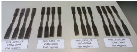
Figure 271 – Coupons extracted from square and rectangular sections after testing
