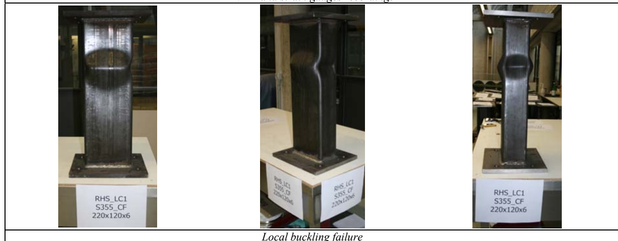
Local buckling failure
