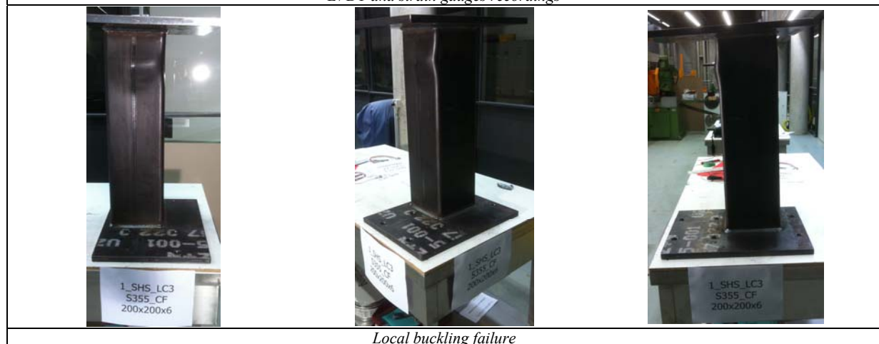
Local buckling failure
