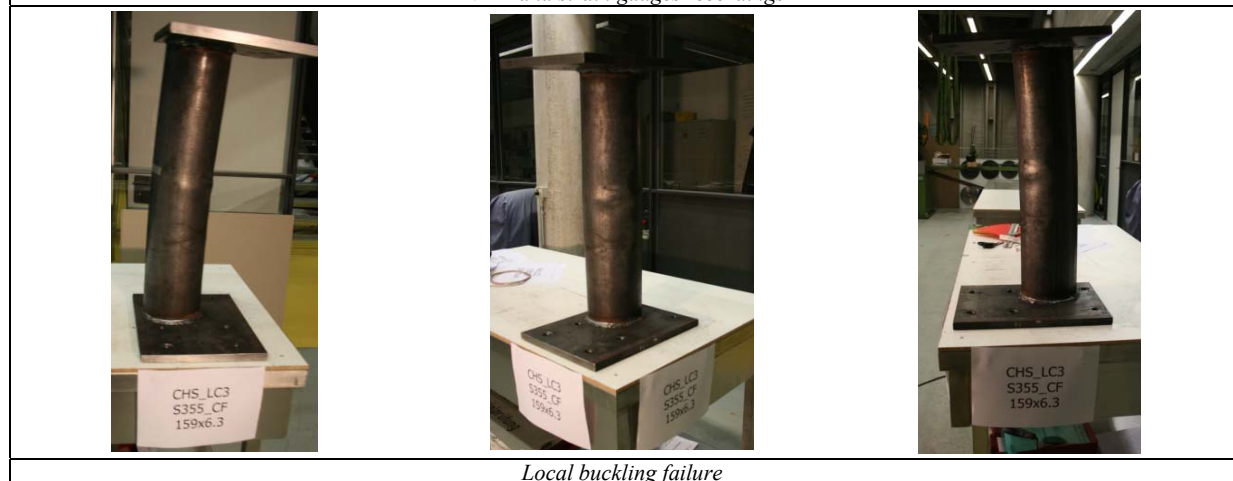
Local buckling failure
