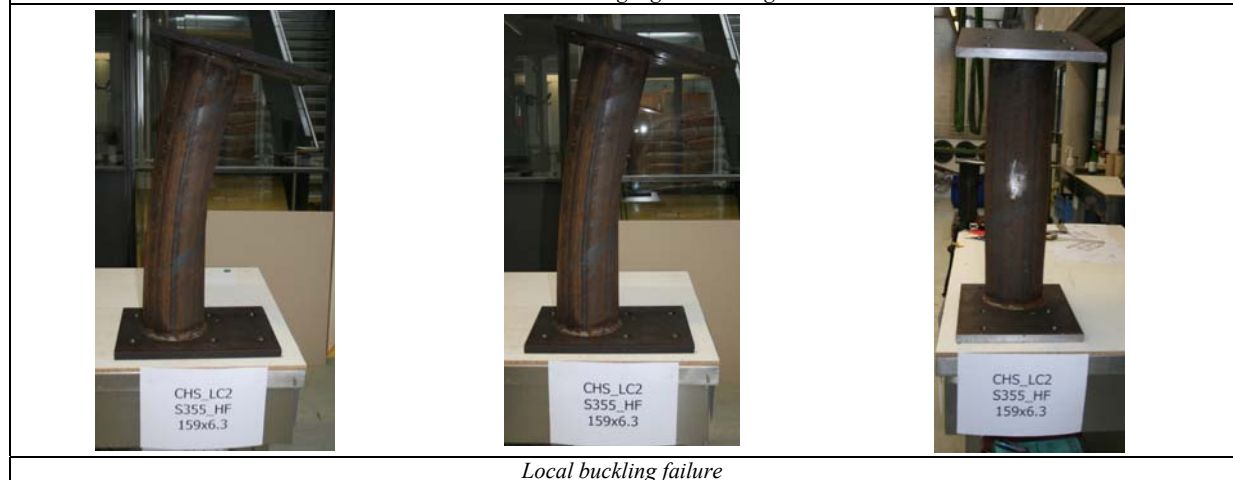
Local buckling failure
