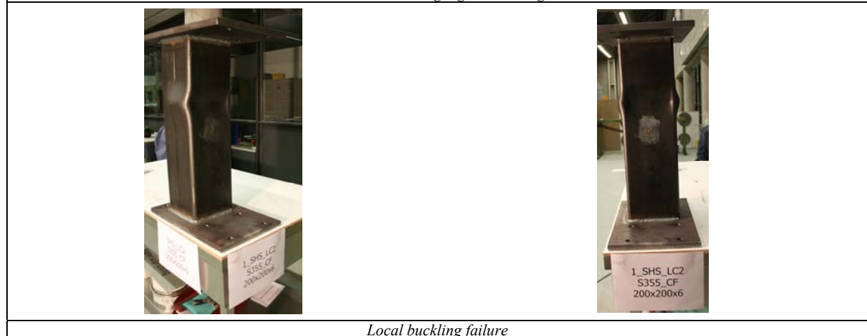
Local buckling failure
