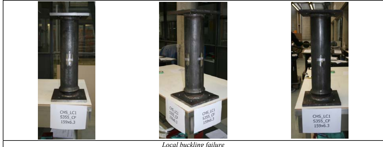
Local buckling failure
