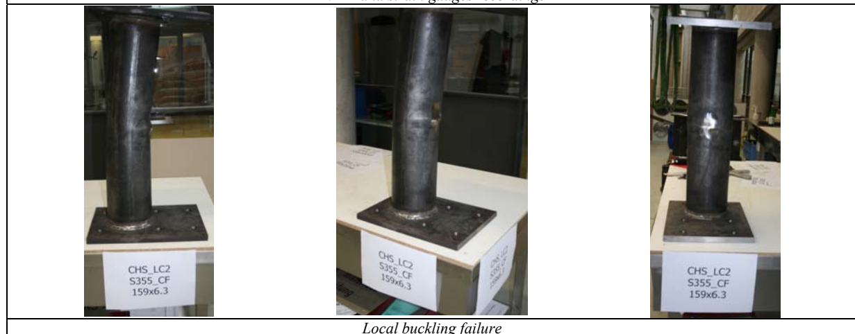
Local buckling failure
