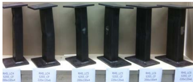
Figure 85 – Failure shapes of all cross-section tests.
