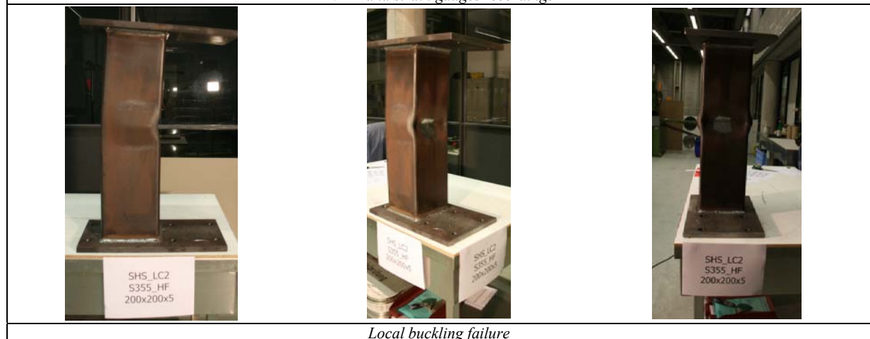
Local buckling failure
