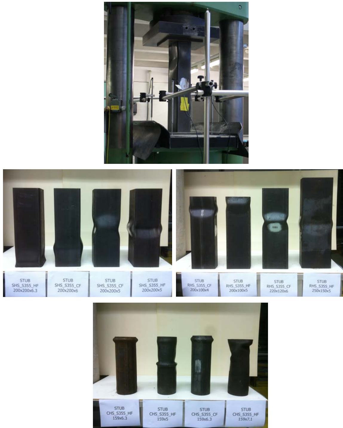
Figure 75 – General test setup and failure shapes of the stub columns.
