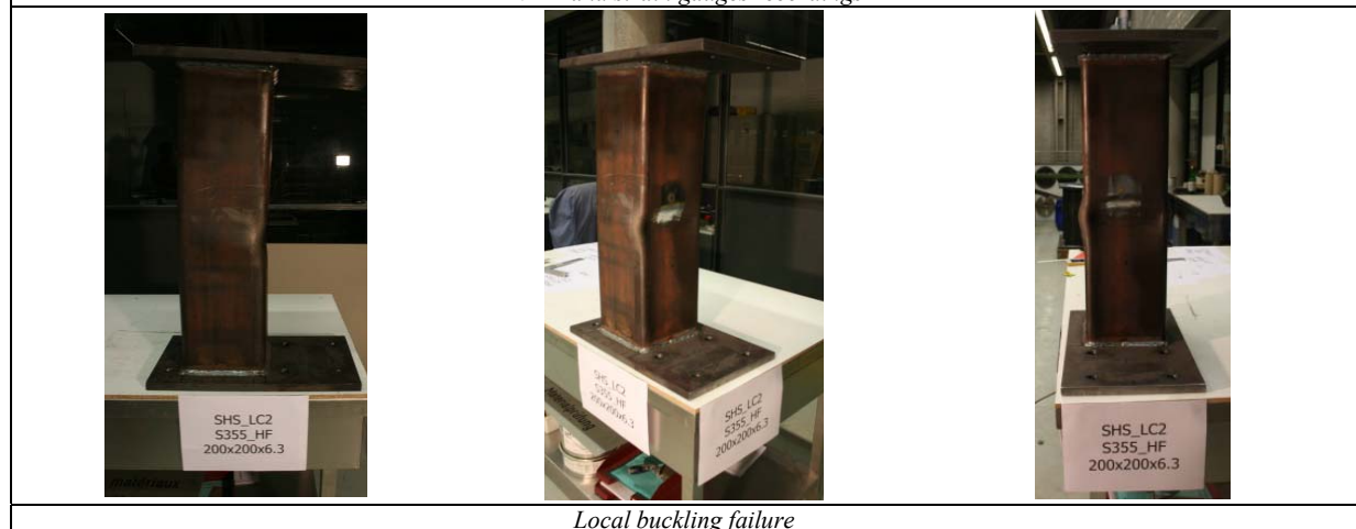
Local buckling failure
