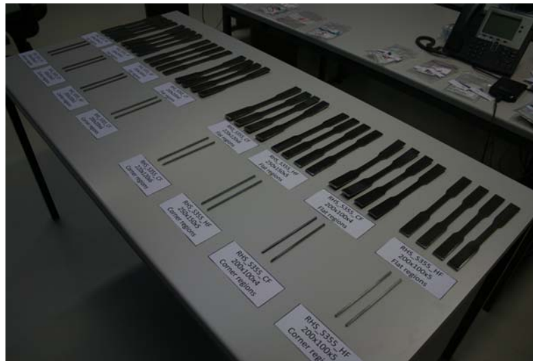
Figure 267 – Test setup and coupons before failure
