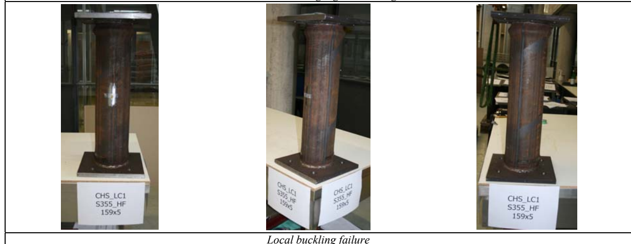
Local buckling failure
