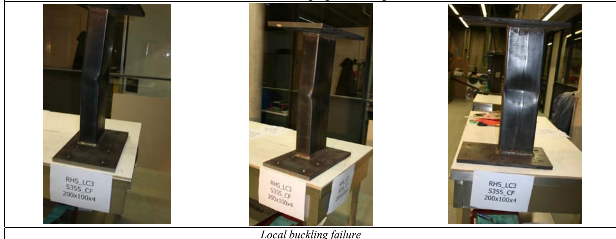
Local buckling failure
