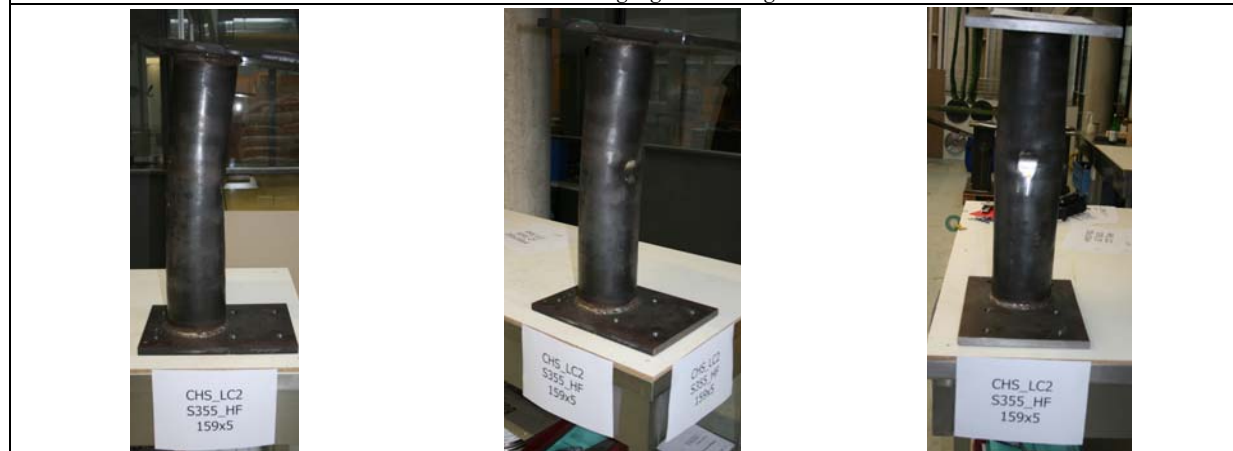
Local buckling failure
