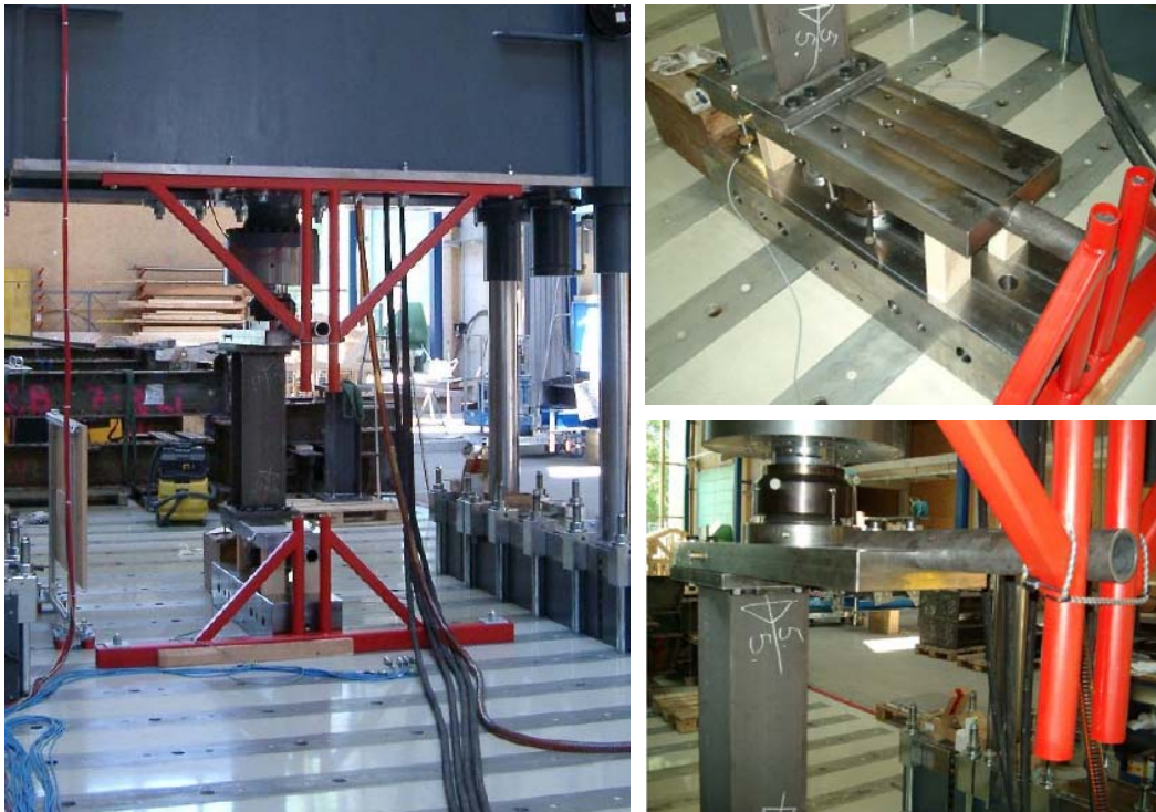
Figure 109 – Testing rig and torsional restraints of loading points of the specimen [7].
