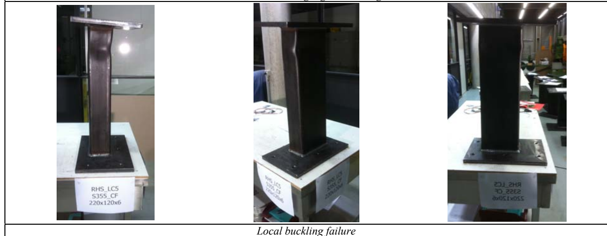
Local buckling failure
