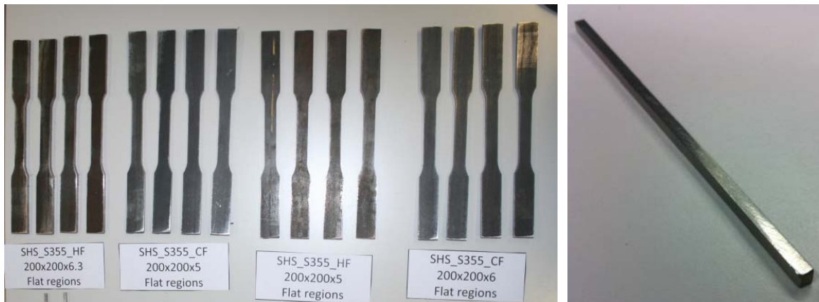
Figure 71 – Necked and straight tensile coupons.
