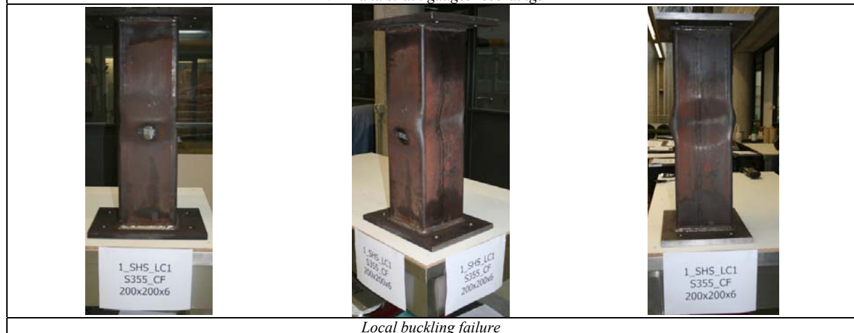
Local buckling failure
