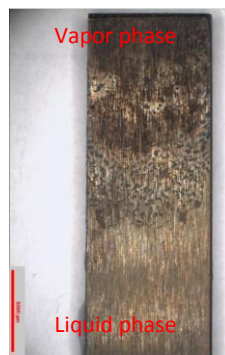
Figure 10: Sample partially immersed in the salt
