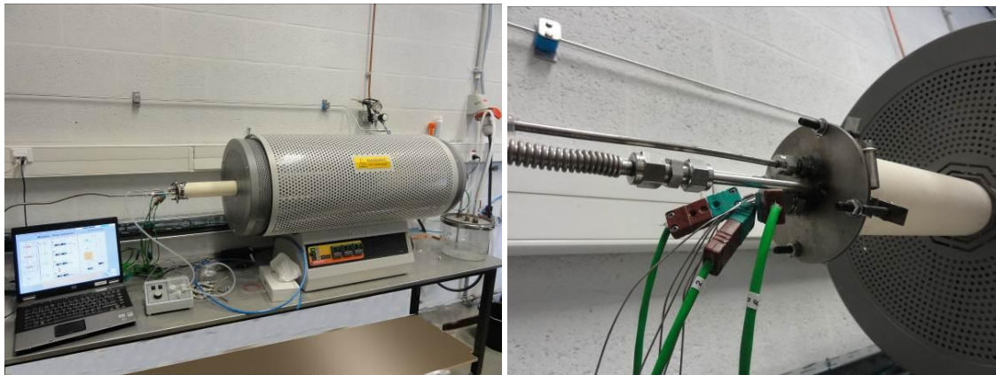
Figure 1: Tubular furnace and instrumentation
