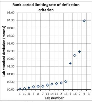
(Filled markers locates test on L<sub>sup</sub>=5200 mm)
