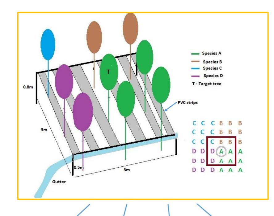
Figure 3: Sketch of a 3m×3m rainout shelter. The frame will be made of wood and about 50% rainfall will be cut off by PVC gutters.
