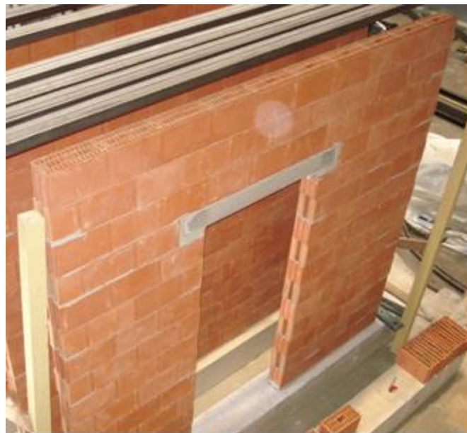
Figure 3: Clay masonry frame test specimen.
