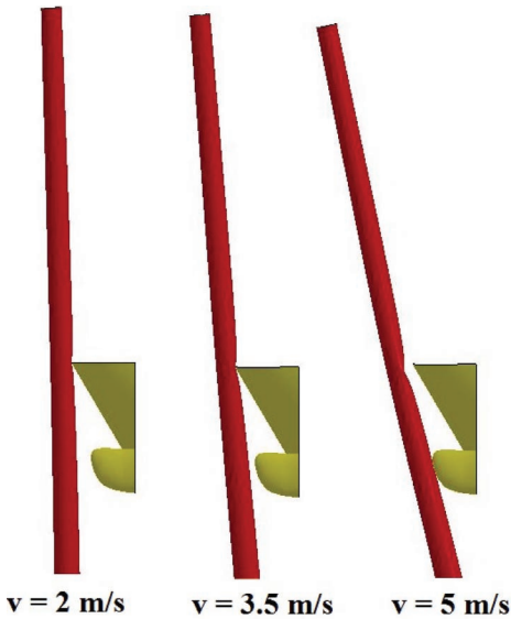
Figure 1. Deformed shape of the structure due to collision.
