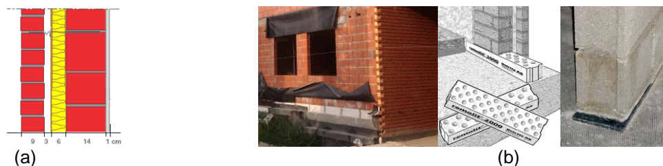
Figure 1. (a) Configuration of a masonry wall in Belgium ; (b) Thermal cut with AAC blocks (left) or foamglass (middle) and acoustic cut with rubber (left)
