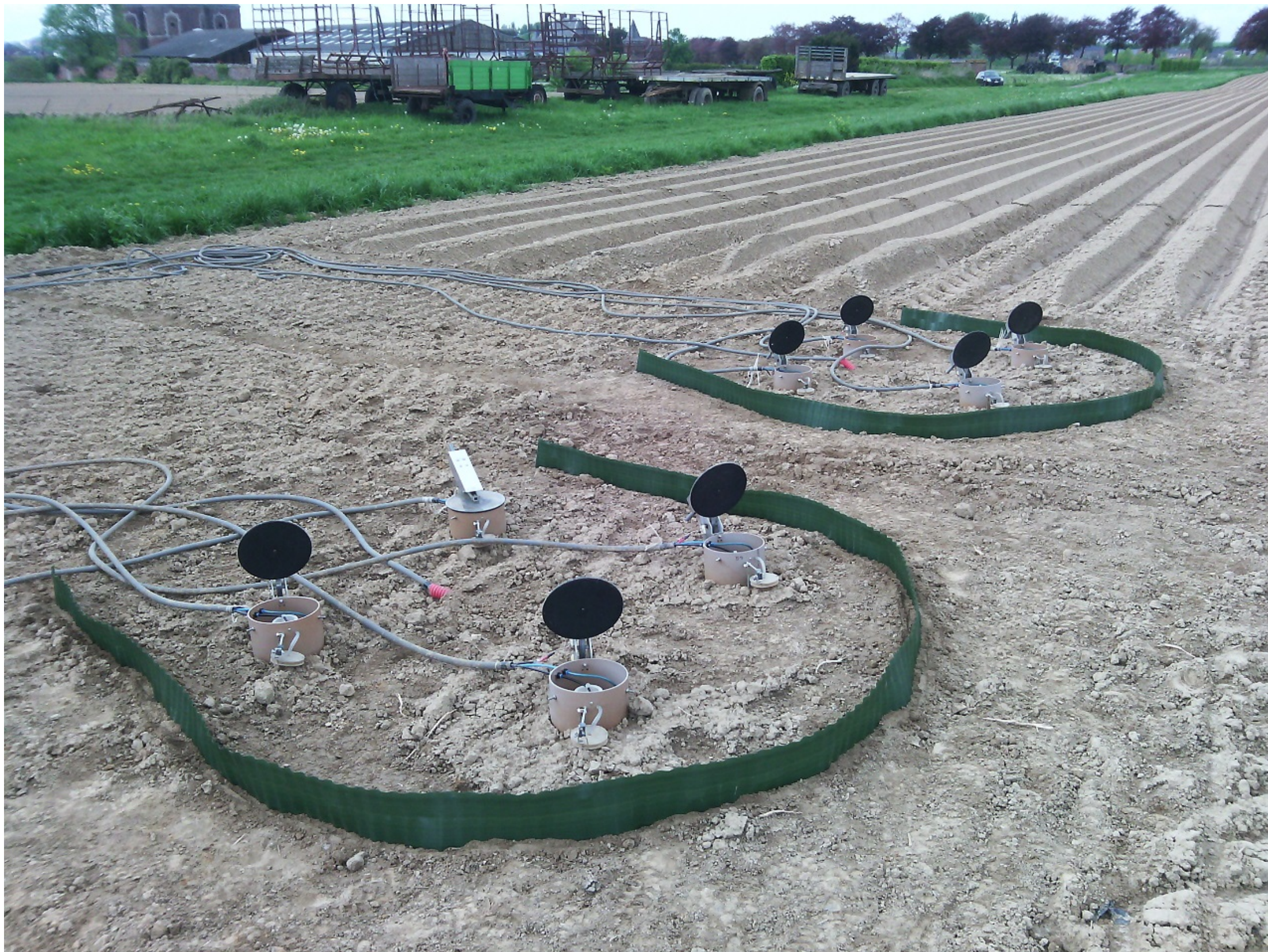
Fig.1 : Experimental setup made of eight chambers. The closed chamber is the one in which N 2 O concentration is measured during the enclosure period, then this chamber reopens and the following chamber is closed.
