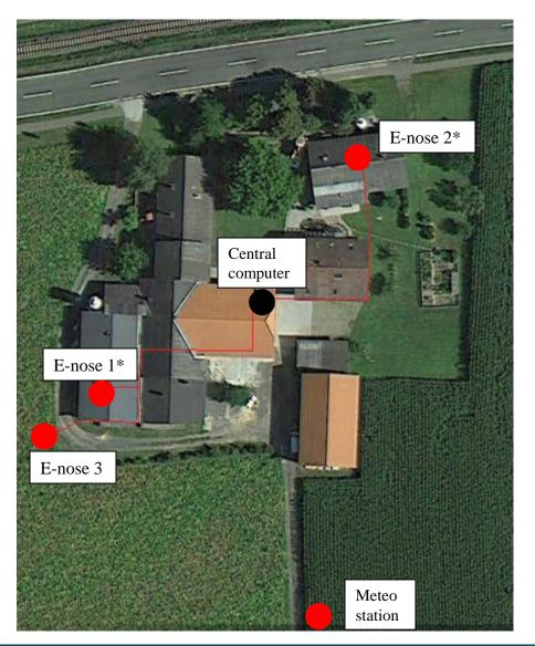
E-nose 1 and 2 : odour and flow monitoring into the stacks → monitoring of all odour emissions from the pig farm.
